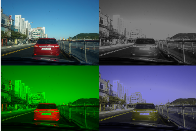
Fig. 2: A scene and the corresponding Lum, RG and BY aspects. The Lum, RG and BY maps are generated by opponent channel encoding.
