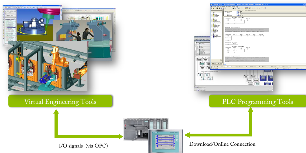
Figure 2-14 Virtual commissioning of a manufacturing cell
