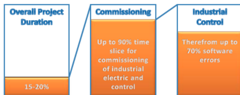
Figure 2-8 Contribution of control software errors to project delay [23]
