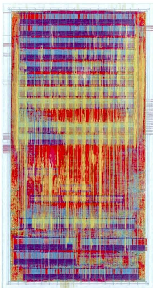
Figure 7-13: Layout for the whole vector processor (vector datapath and VLSU unit)
