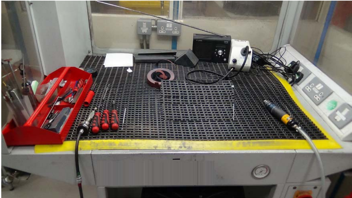
Figure 5-2. Manual de-burring process working-cell
