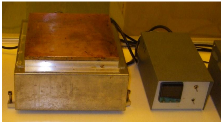
Figure 5.82: The hot plate and temperature control unit used in this manufacturing approach.
