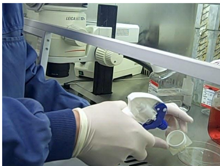
Figure 6.13: Sterilisation procedure for the first batch of tests, soaking in industrial methylated spirit (IMS).
