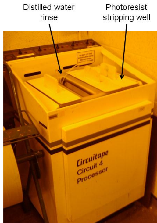
Figure 5.40: The Circuitape Circuit 4 Processor used for photoresist stripping following Cu etching.
