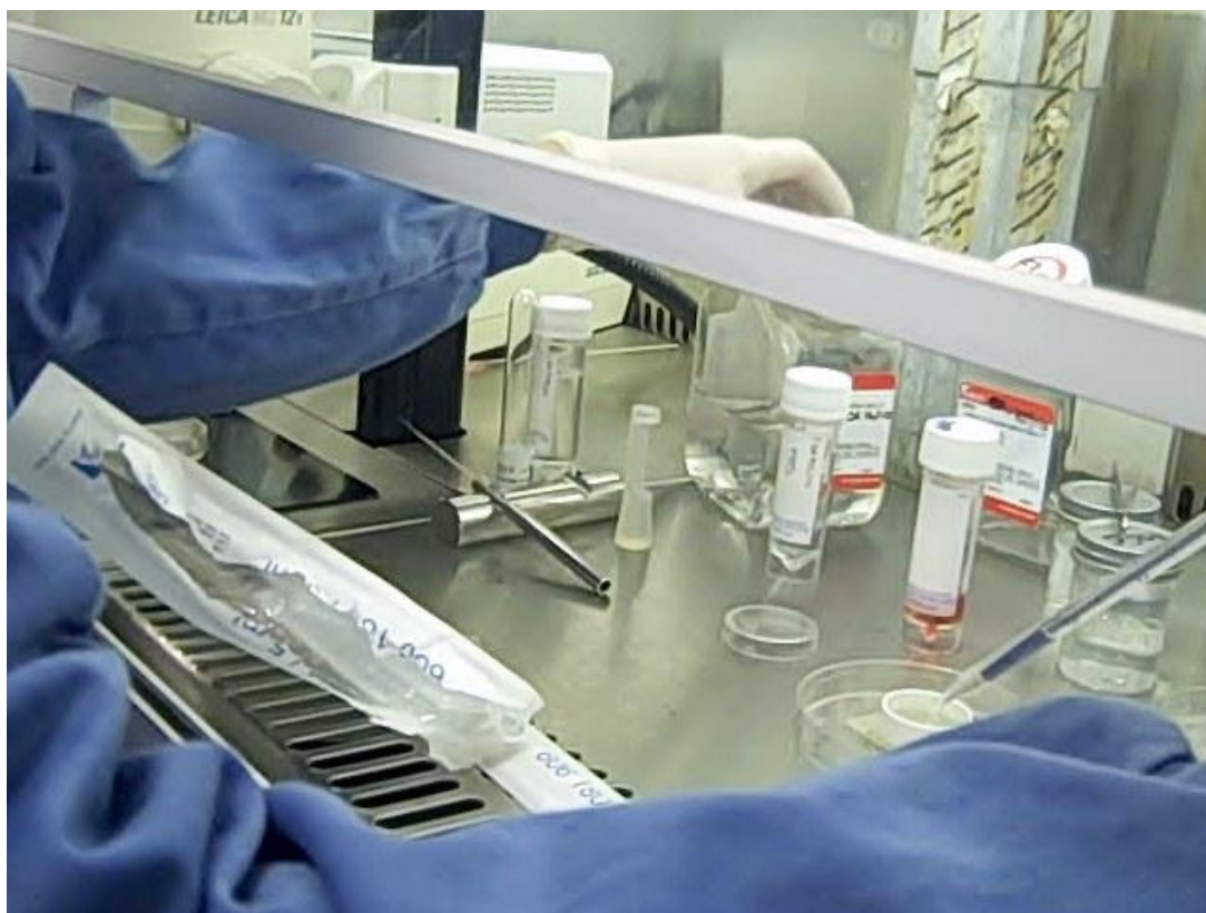
Figure 6.15: MEA biochip is rinsed with phosphate buffered solution (PBS).
