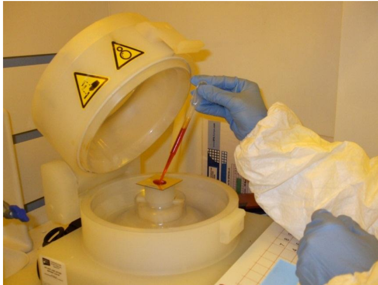
Figure 5.81: Application of AZ 9260 onto a Ti/Au coated base substrate.
