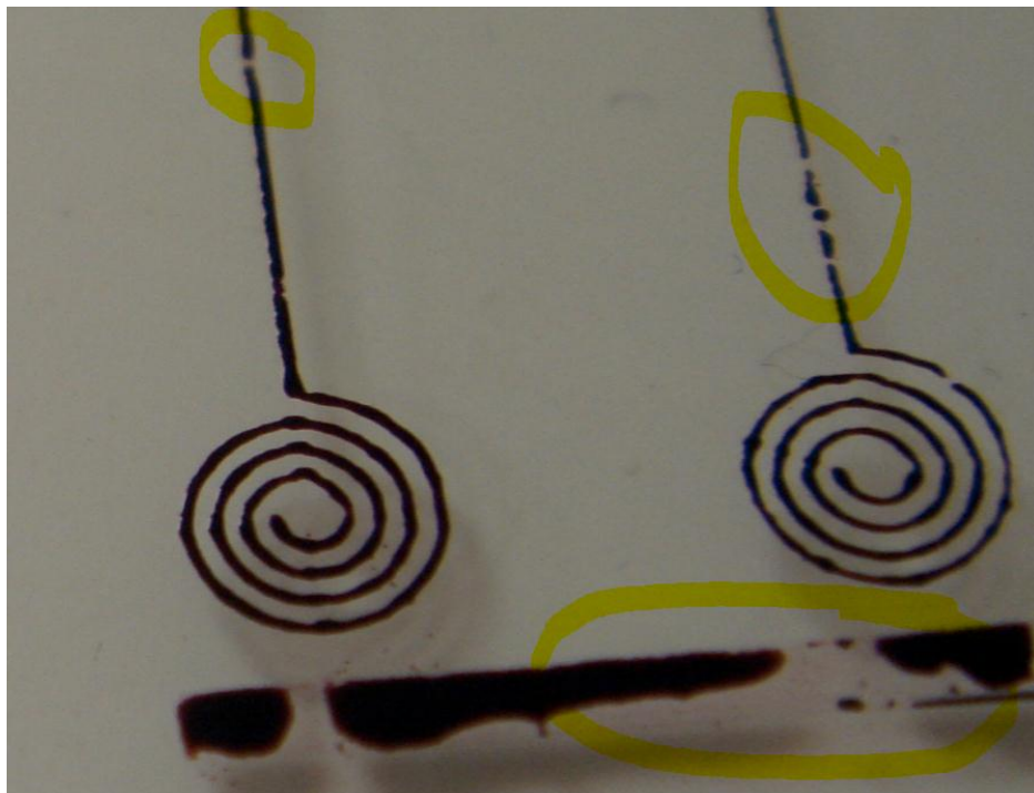
Figure 5.94: Examples of the failed adhesion (highlighted within yellow circles) of the Au ink to the surface of the glass.
