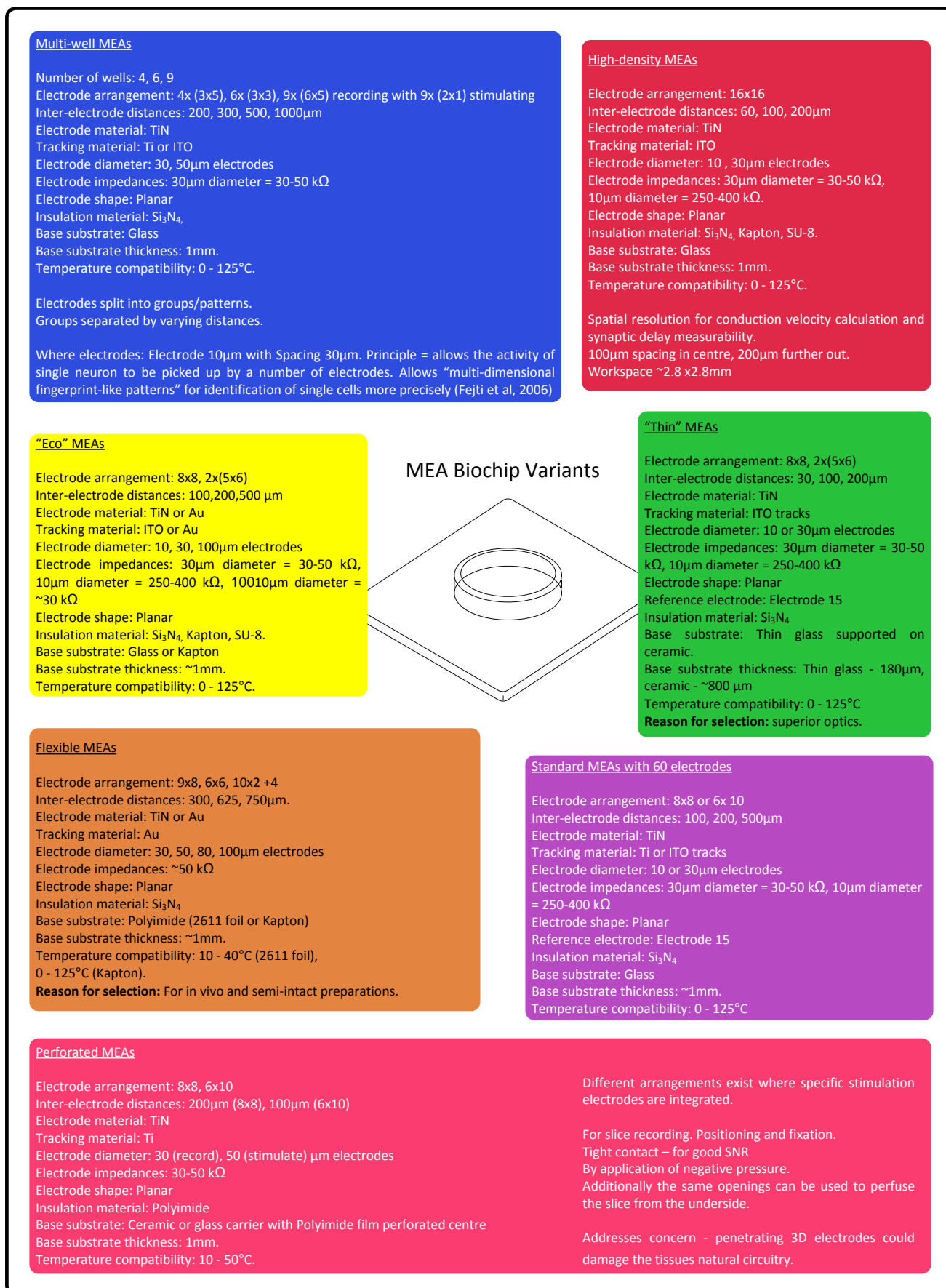
Figure 2.65: A summary of state-of-the-art commercially available MEA biochips. Microelectrode shapes, materials, diameters, impedances and temperature compatibility can all be compared quickly.
