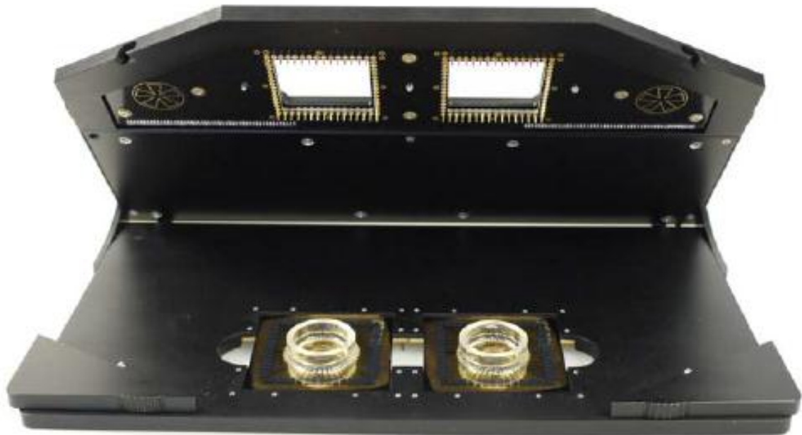
B.1: The two available variants of the MEA2100 headstage.
