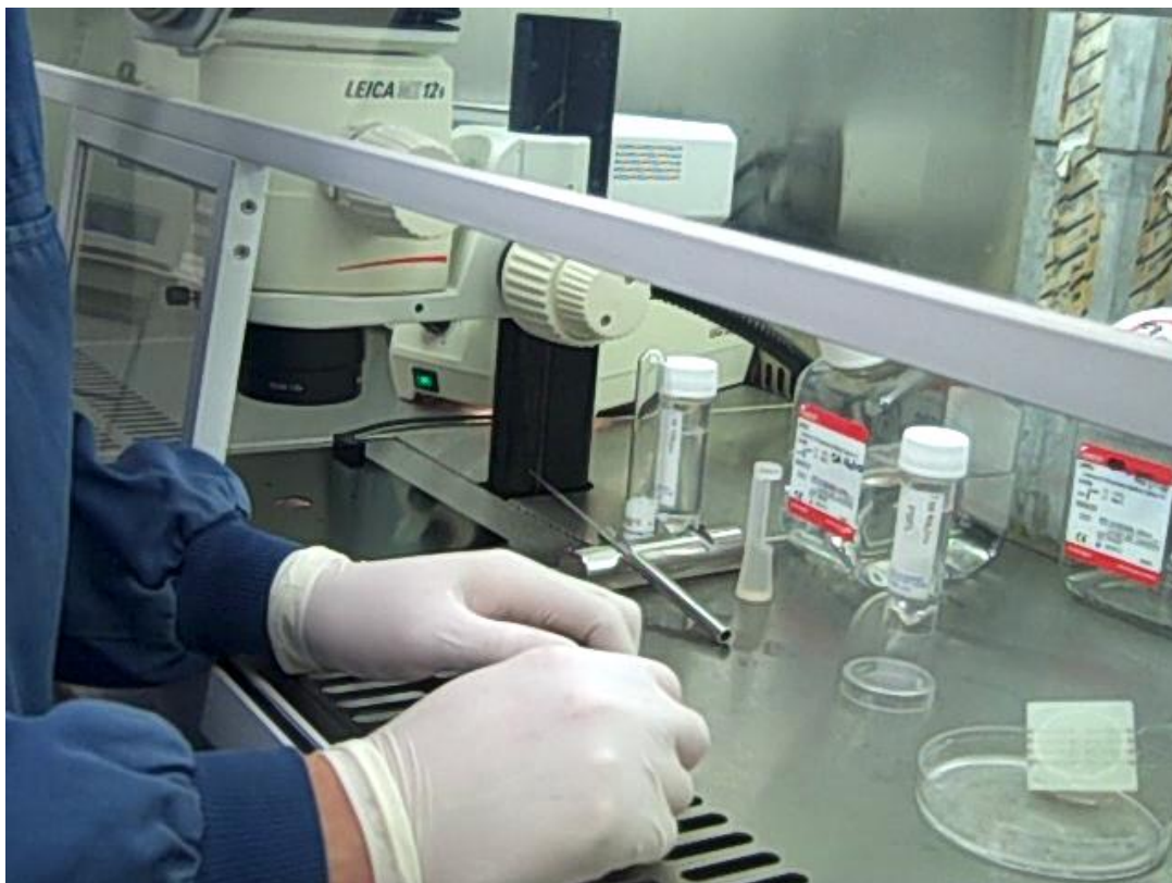
Figure 6.14: MEA biochip is left to dry inside the laminar flow culture hood.
