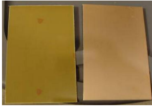
Figure 5.19: Copper laminated FR4 used as base substrate for manufacturing approaches 1, 2 and 3, and consequently Prototype 1.
