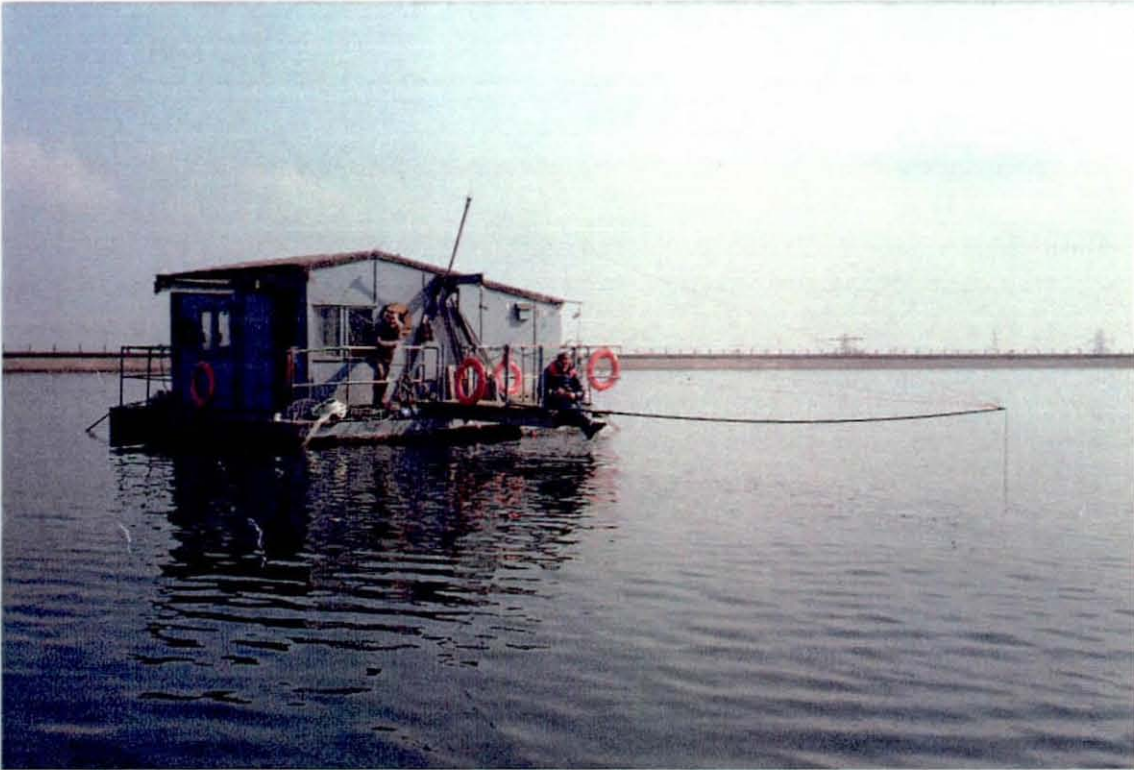
Fig.5.2/1 Trials facility at Staines Reservoir. - Hydrophone support pole deployed.
