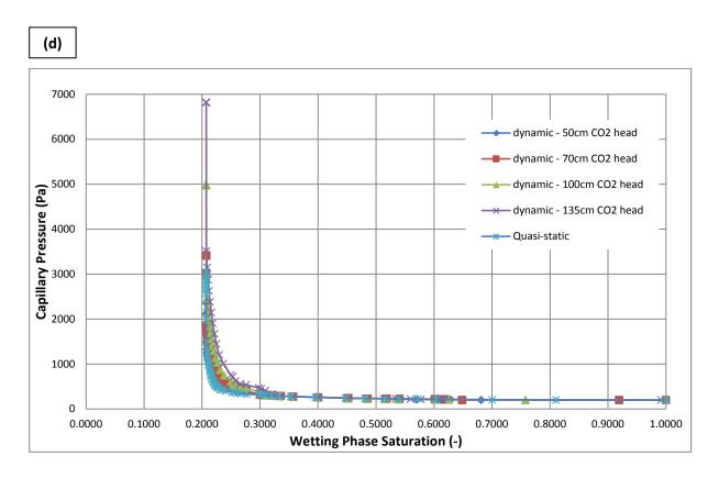
Figure 2. Dynamic and Quasi-Static Capillary Pressure – Saturation Curves for Coarse Sand at (a)  $35^{\circ}$ C, (b)  $45^{\circ}$ C, (c)  $55^{\circ}$ C and (d)  $65^{\circ}$ C. These curves are based on porous medium properties obtained from experimental measurements (Table 6).
