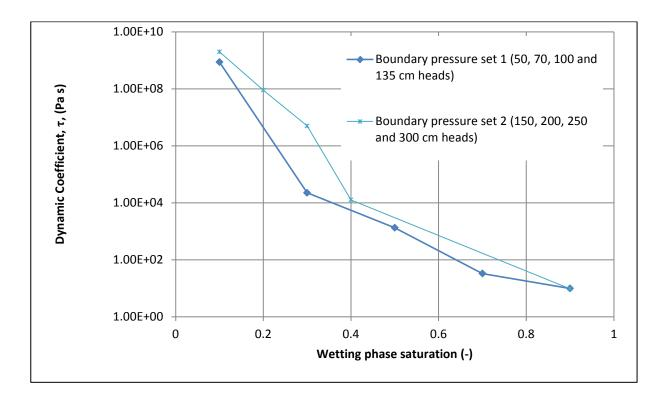
Figure 10: Dynamic coefficients from different set of boundary conditions. Please note that boundary pressure set 1 was applied in all other results in this paper including grid convergence test (Figures 1 – 9). These semi-log plots are based on porous medium properties obtained from experimental measurements (Table 6).
