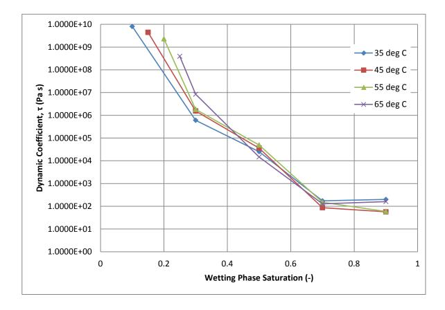
Figure 7: Dynamic Coefficients in Fine Sand at Different Temperatures. These semi-log plots are based on porous medium properties obtained from experimental measurements (Table 6).
