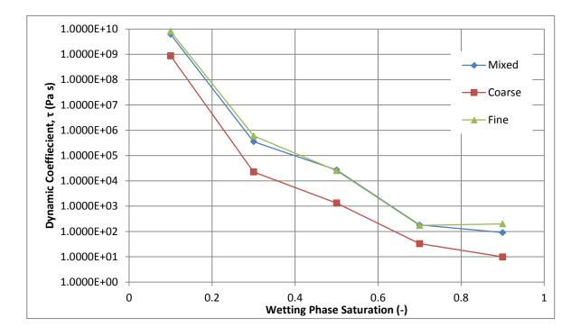
Figure 9: Dynamic Coefficients in Coarse, Fine and Mixed Sand Samples at 35°C. These semi-log plots are based on porous medium properties obtained from experimental measurements (Table 6).
