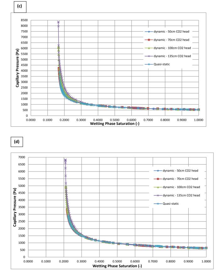
Figure 3. Dynamic and Quasi-Static Capillary Pressure – Saturation Curves for Fine Sand at (a)  $35^{\circ}$ C, (b)  $45^{\circ}$ C, (c)  $55^{\circ}$ C and (d)  $65^{\circ}$ C. These curves are based on porous medium properties obtained from experimental measurements (Table 6).
