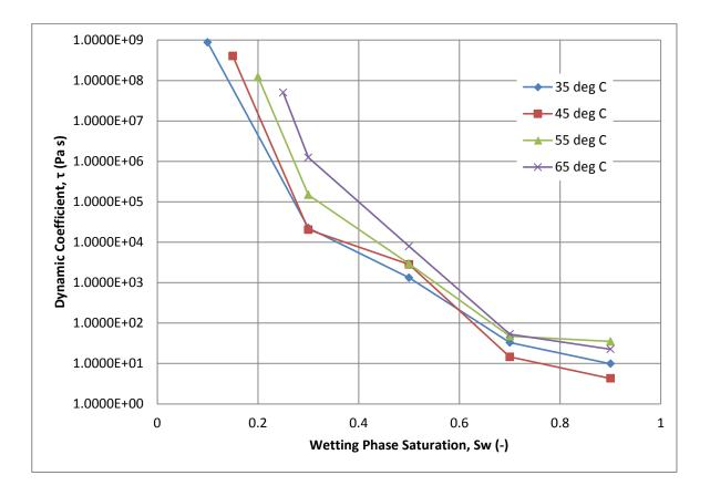
Figure 6: Dynamic Coefficients in Coarse Sand at Different Temperatures. These semi-log plots are based on porous medium properties obtained from experimental measurements (Table 6).
