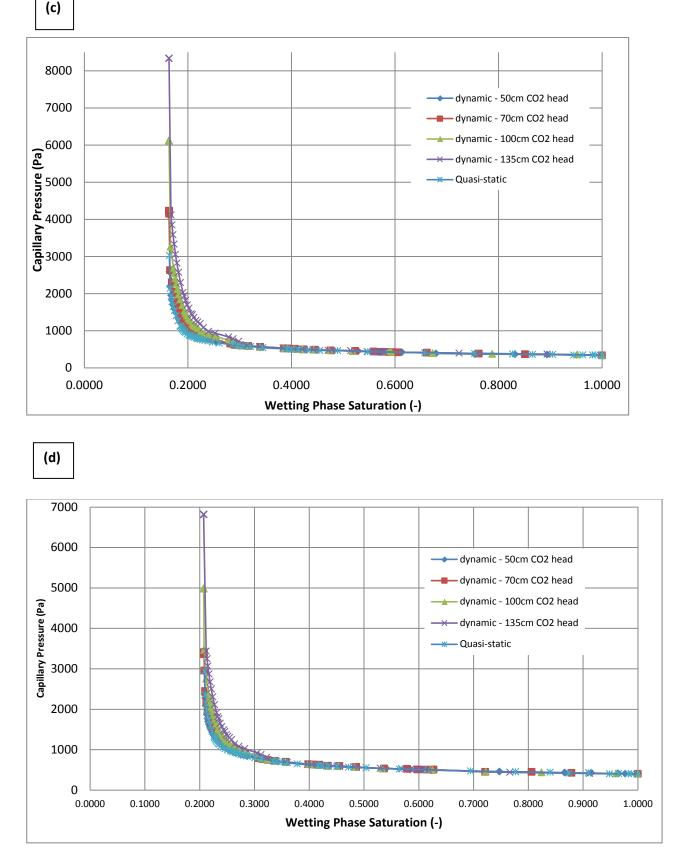
Figure 4. Dynamic and Quasi-Static Capillary Pressure – Saturation Curves for 50% Fine Sand and 50% Coarse Sand Mixture at (a)  $35^{\circ}$ C, (b)  $45^{\circ}$ C, (c)  $55^{\circ}$ C and (d)  $65^{\circ}$ C. These curves are based on porous medium properties obtained from experimental measurements (Table 6).
