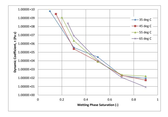
Figure 8: Dynamic Coefficients in Mixed Sand Sample at Different Temperatures. These semi-log plots are based on porous medium properties obtained from experimental measurements (Table 6).
