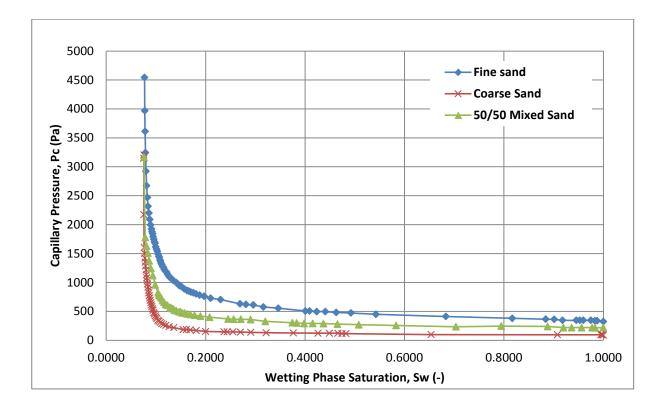
Figure 5. Comparison of Quasi-Static Capillary Pressure–Saturation Curves for Fine Sand, Coarse Sand and 50% Fine Sand and 50% Coarse Sand Mixture at 35<sup>o</sup>C. These curves are based on porous medium properties obtained from experimental measurements (Table 6).
