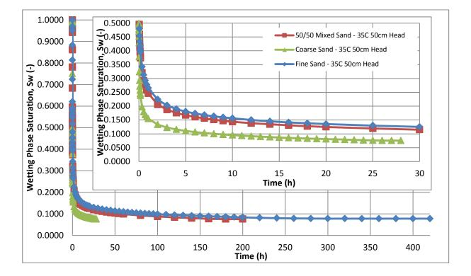
Figure 1. Saturation-Time curves for Coarse Sand, Fine Sand and Mixed Sand, all obtained at 35<sup>o</sup>C and pressure heads of 50 cm. These curves are based on porous medium properties obtained from experimental measurements (Table 6).
