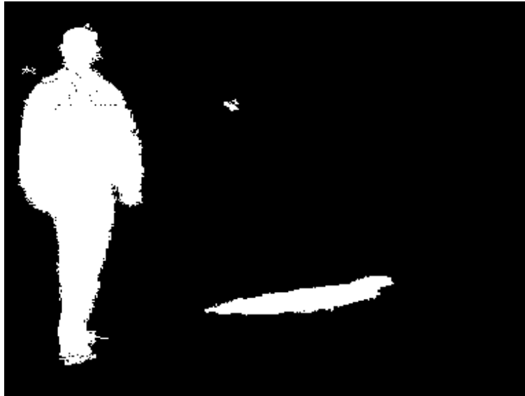
Fig. 2.9 – Thresh_Sizefilt249 is Thresh249 in Fig. 2.3c after applying the size filter. Almost all spurious pixels less than T_0 (e.g. T_0 = 10 ) have been removed from the thresholded image using a simple size filter. Meanwhile, the shapes of foreground objects have not been distorted.
