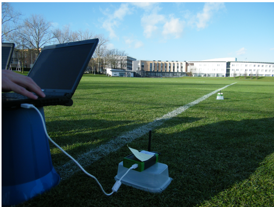
Figure 6.3: Transmission range measurement setup.
