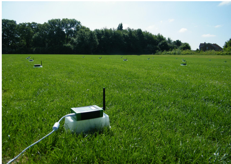
Figure 6.13: The large WSN testbed deployment on a field.
