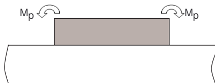
Figure 2.3: PZT patch actuator
