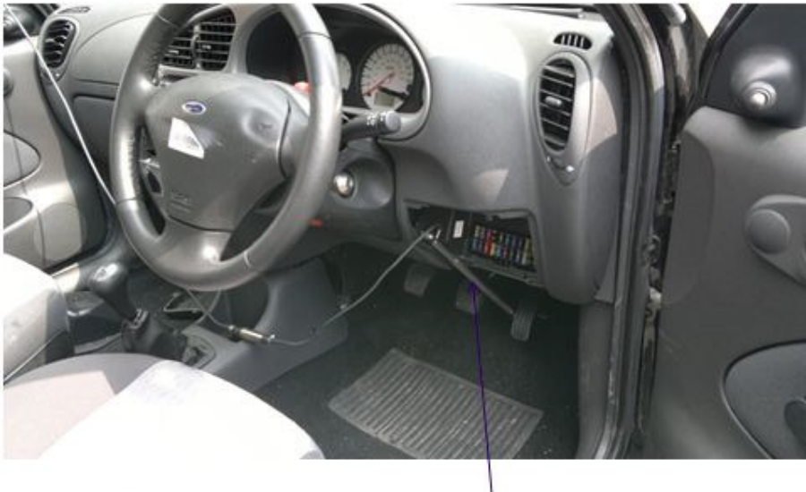
Linear potentiometer fitted to measure accelerator pedal travel
