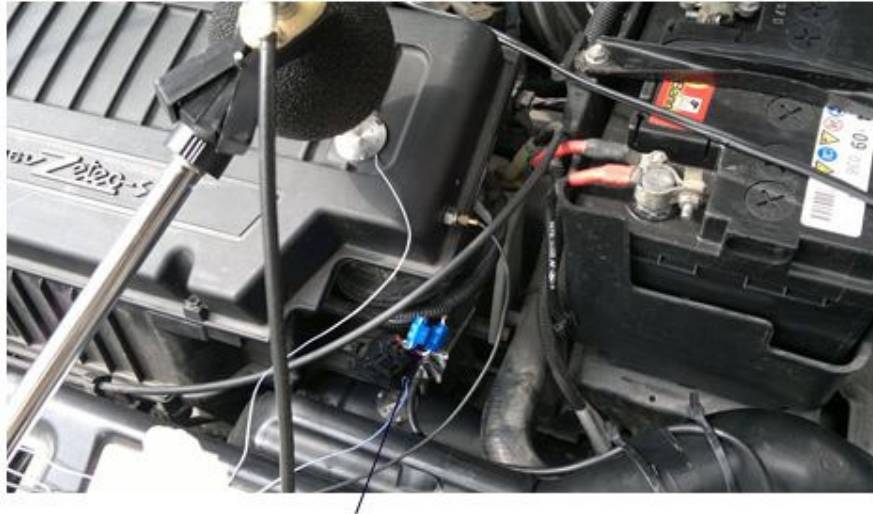
Electrical connection taken from the wire of throttle body to measure throttle angle
