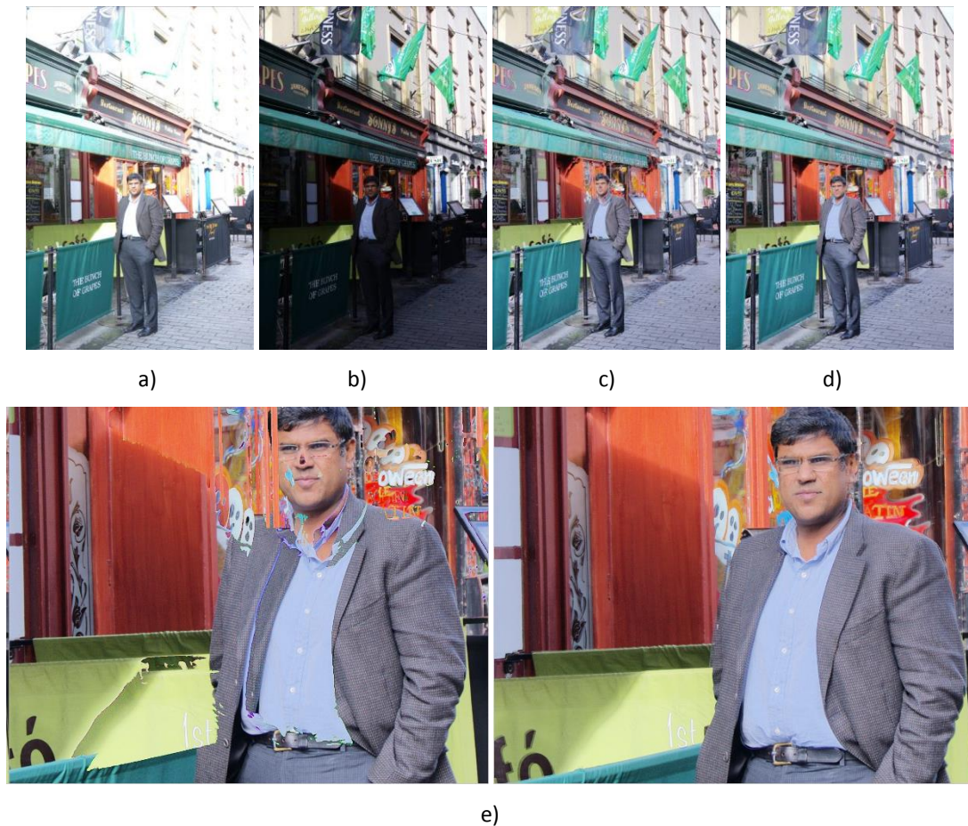
Figure 5.9: Ability of the proposed method to compensate for motion. a) and b) shows the over and under exposed images. c) The fused image without motion compensation. d) The fused image with motion compensation enabled. e) Zoomed in crops of (c) and (d).
