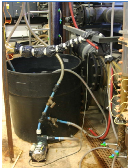
Figure 63 - Raw water storage tank showing delivery pump and mixing system
