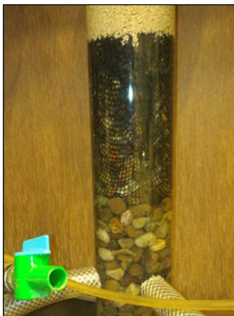
Figure 61 - Supporting media in laboratory filter columns
