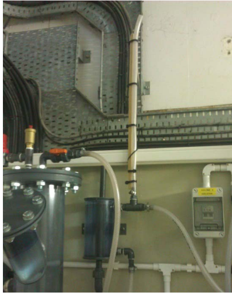
Figure 92 - Re-design of de-bubbler on pilot plant
