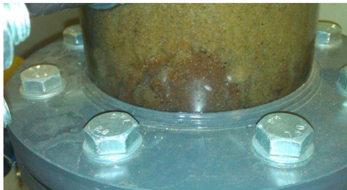
Figure 96 – Mudballs settled at the base of the filter column
