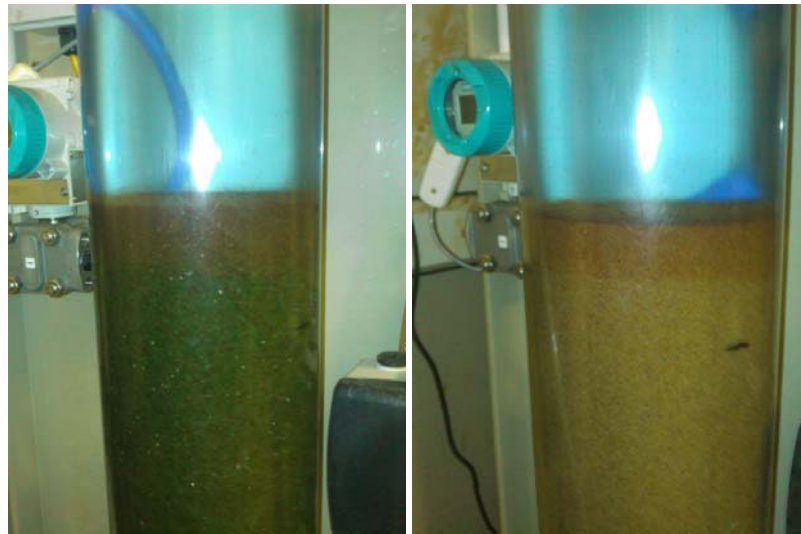
Figure 94 - View of glass and sand saturated by iron in the upper layer, other media are darker and so mat is less visible
