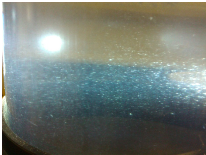
Figure 93 - Floc entering the pilot plant filter columns
