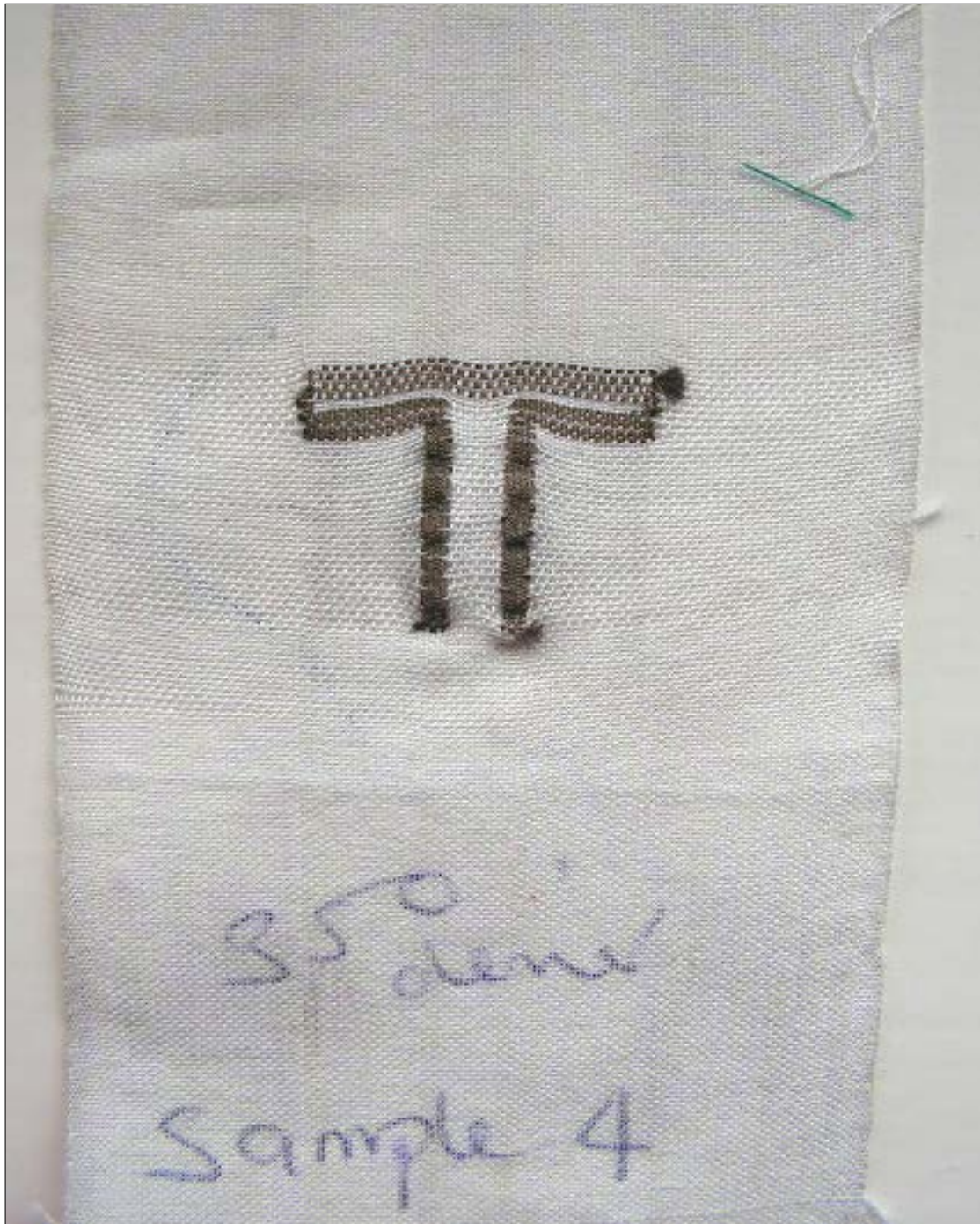
Fig 45 Image of a woven folded dipole antenna using 350 denier X-Static yarn, Authors own photograph
