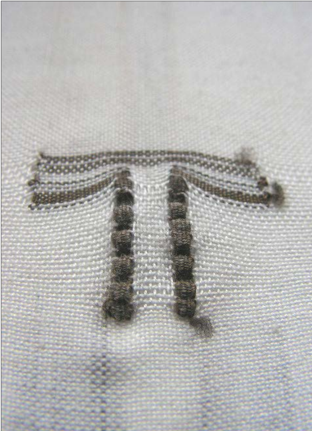
Fig 47 Close up image of woven folded dipole antenna illustrating again the raised nature of the X-Static yarn, Authors own photograph
