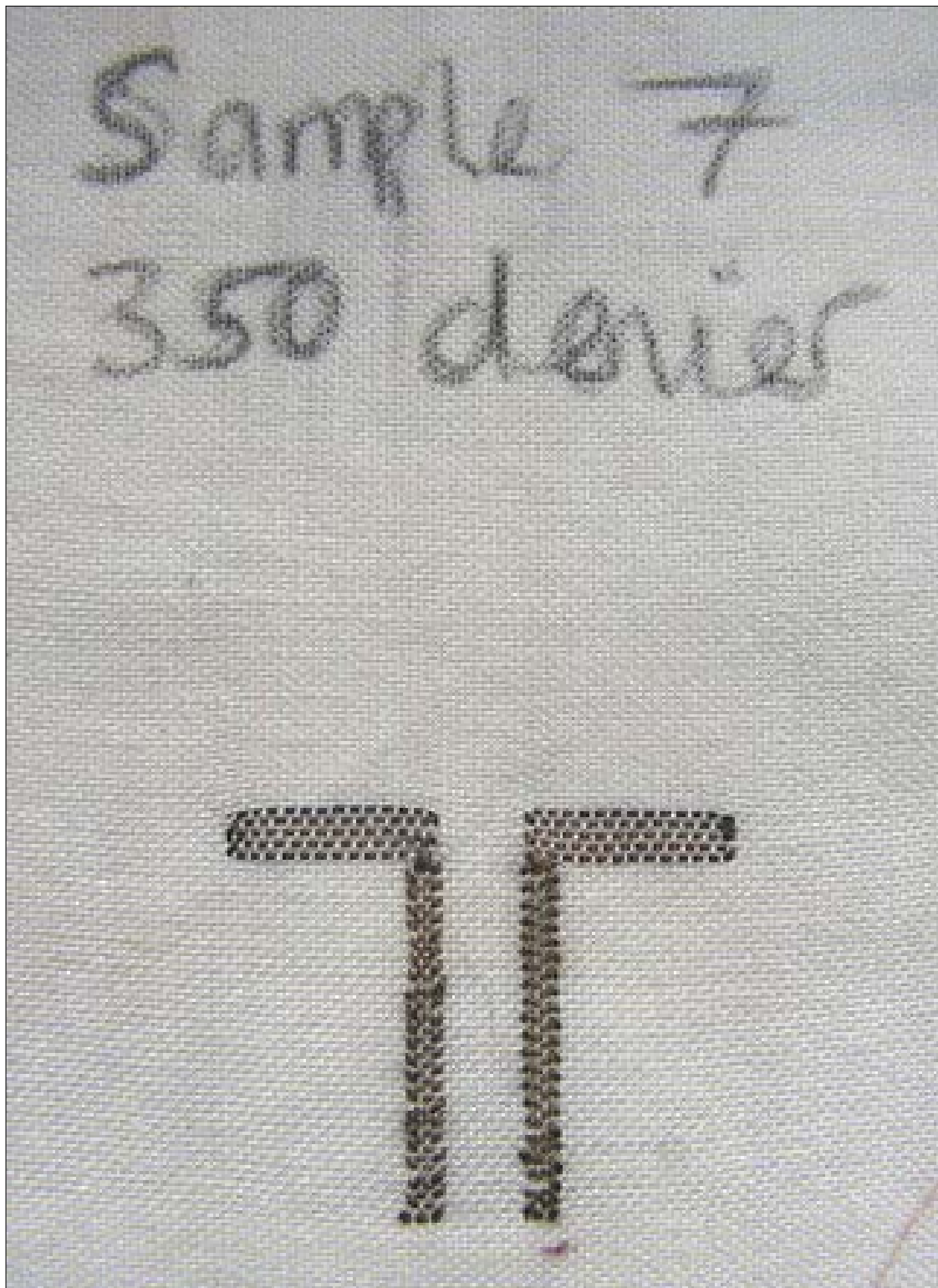
Fig 53 Image of a woven dipole antenna using 350 denier X-Static yarn. Authors own photograph
