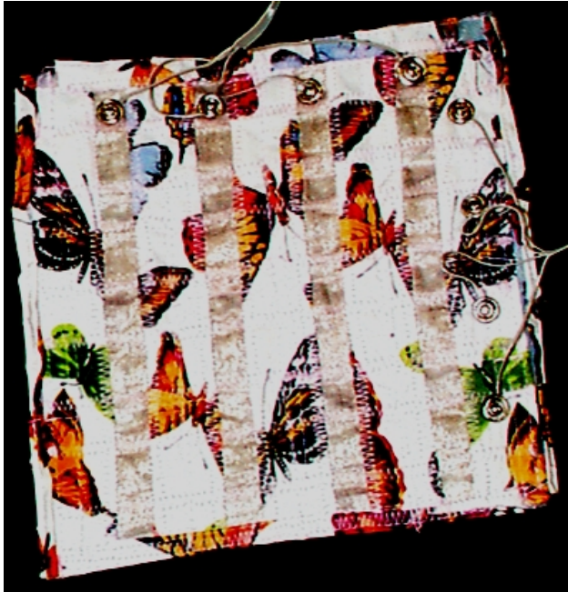
Fig 2 Image of the all fabric keyboard developed at MIT
