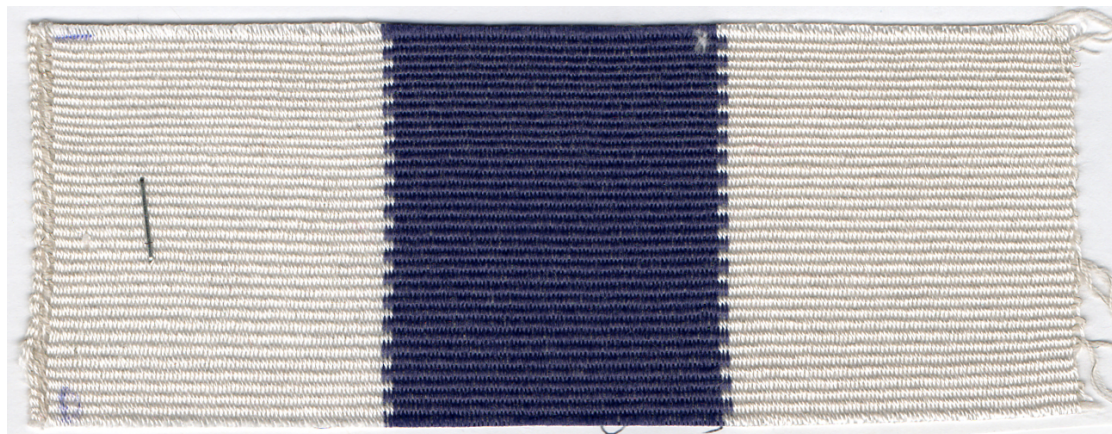
Fig 31 woven sample showing the 3 sections of cloth, on the left is the cotton, central is the polyester and on the right is the tencel
