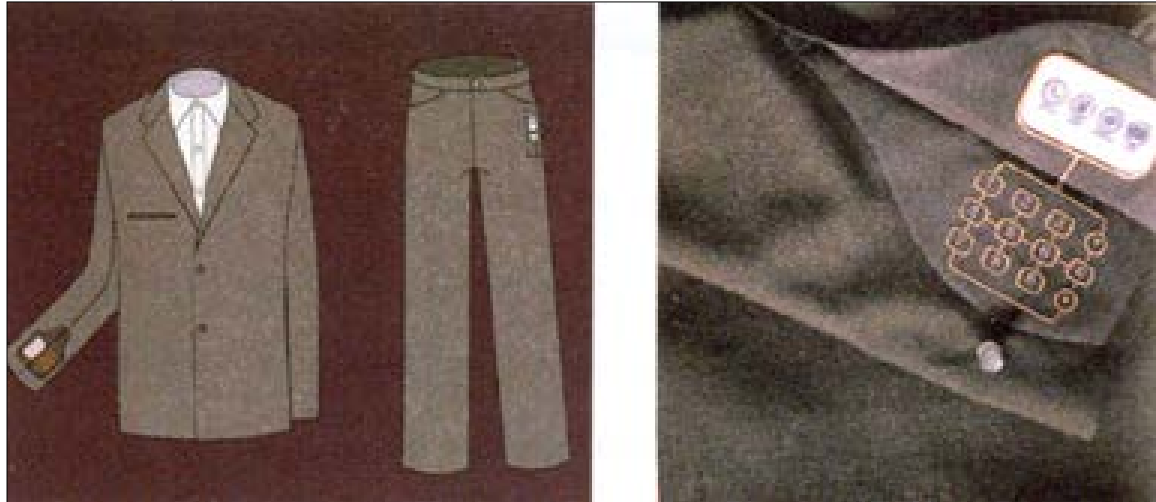
Fig 3 Illustration of the business suit produced by Philips [13] the image on the right shows the embroidered keypad situated under the flap on the cuff
