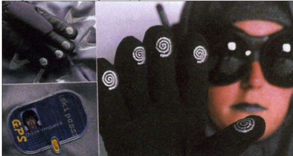
Fig 4 illustration of the snowsuit produced by Philips [13] the printed conductors can be seen on the tips of the gloves, used for activating the MP3 player.
