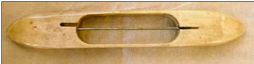
Fig 101 Photograph of a shuttle. Authors own image.
