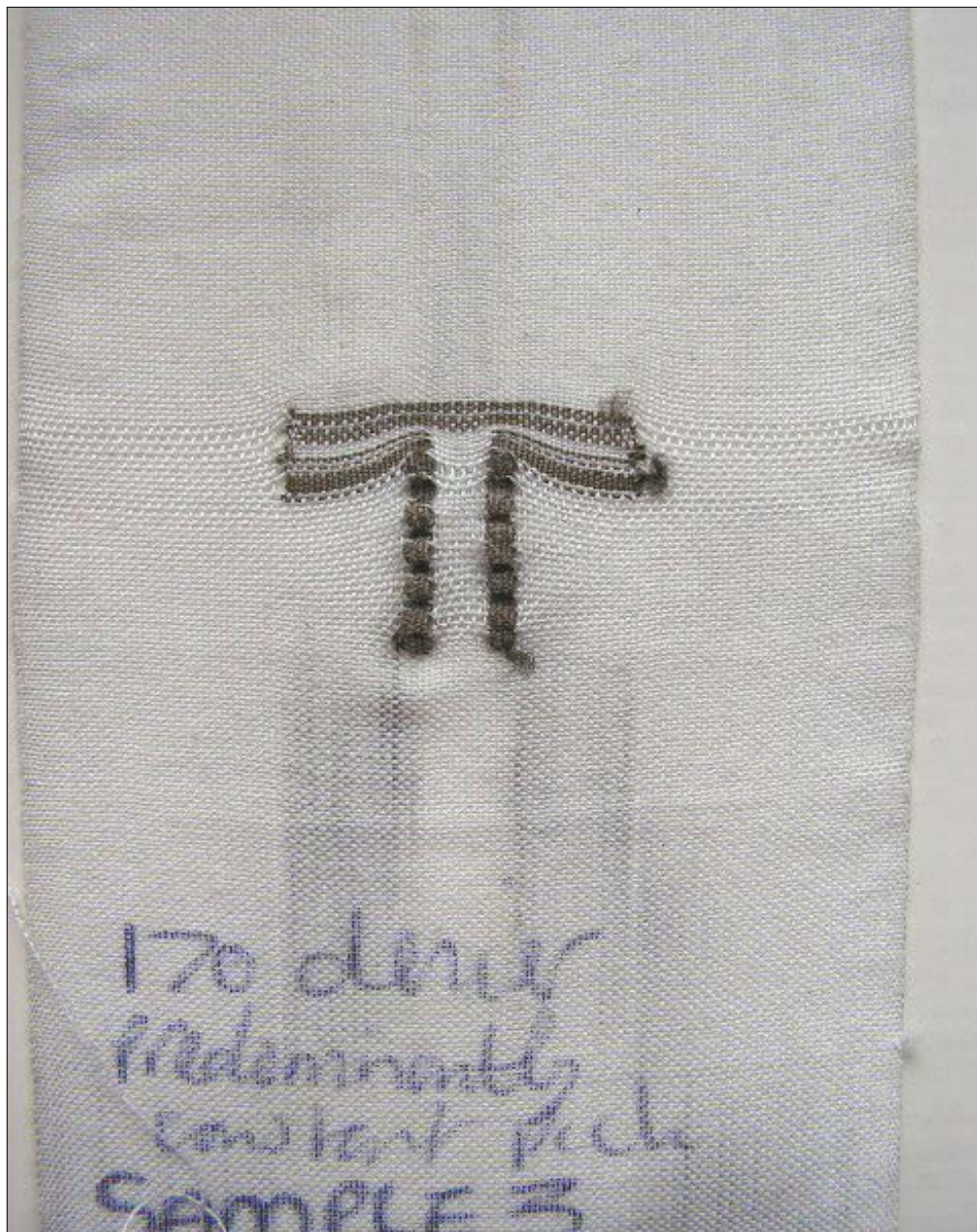
Fig 44 Image of a woven folded dipole antenna using 170 denier X-Static, Authors own photograph
