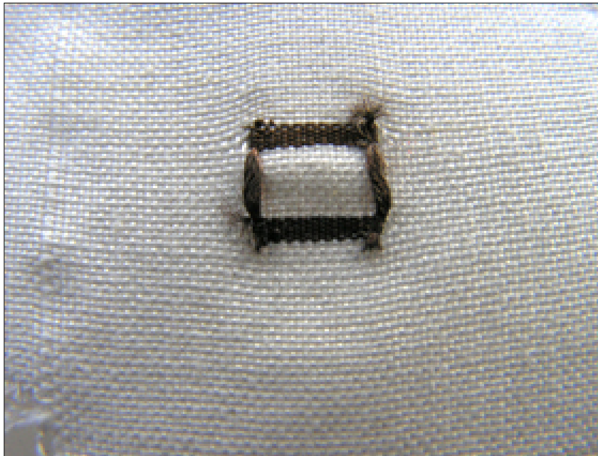
Fig 40 close up of the 26mm conductor loop. The untidy finishing on the warp and weft joins is evident and can be seen where the red circle is indicating.
