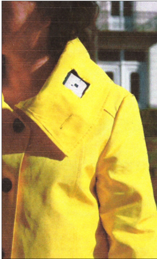
Fig 24 Image showing integrated textile antenna within the collar of a coat [45]
