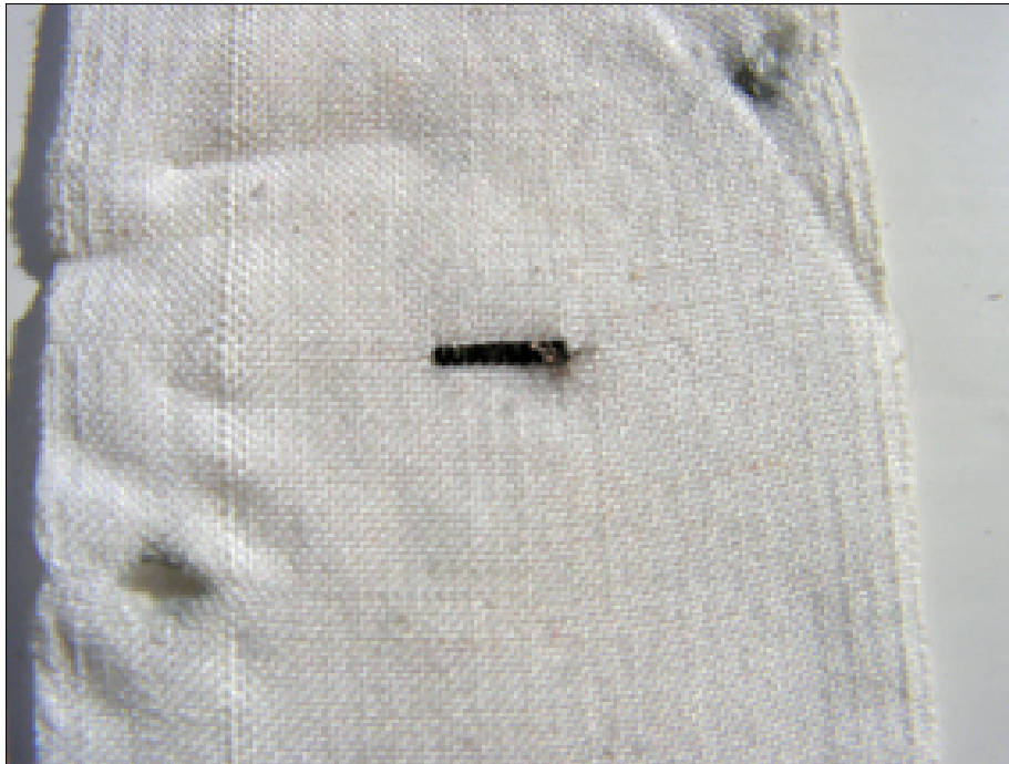
Fig 32 shows the X-Static conductor track and its position in the cloth sample, authors own image
