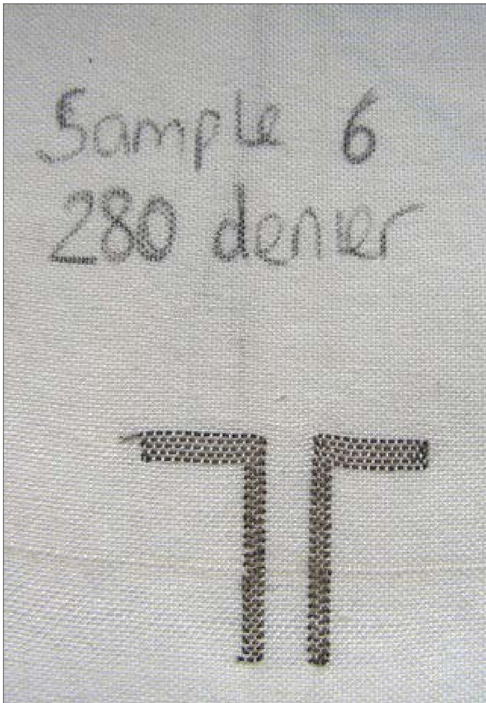
Fig 52 Image of a woven dipole antenna using 280 denier X-Static yarn. Authors own photograph
