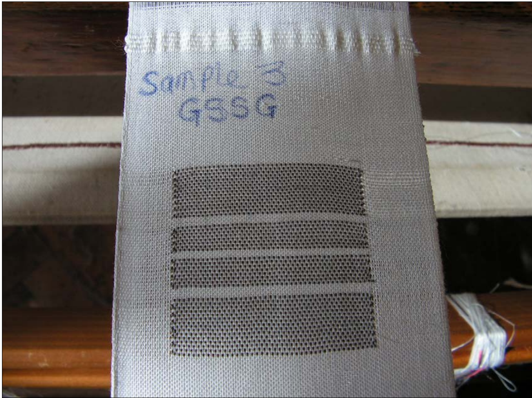
Fig 88 Photograph of woven transmission lines, configuration 3. Authors own photograph
