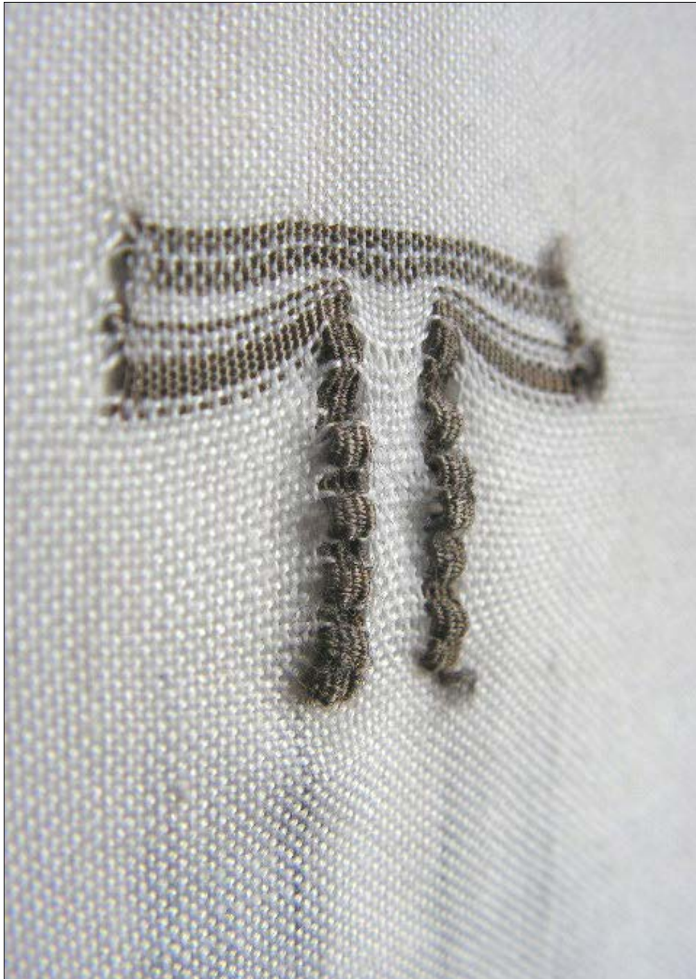
Fig 46 Close up image of Woven folded dipole antenna illustrating the raised nature of the yarn. Authors own photograph
