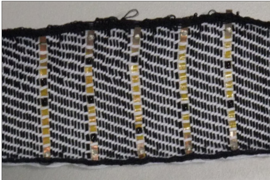
Fig 26 photograph of conductive yarn and plastic fibres integrated into a woven fabric
