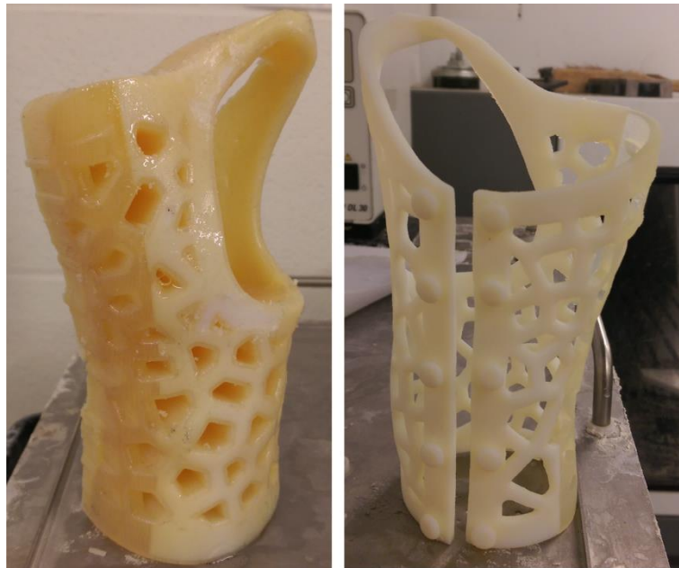
Figure 8. Physical prototype of the AM splint: As is after the printing process (left) and after post-processing (right).
