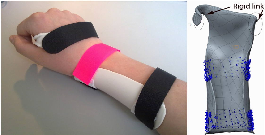
Figure 5. Velcro strips (left) and modelled constraints (right) for the classic splint.
