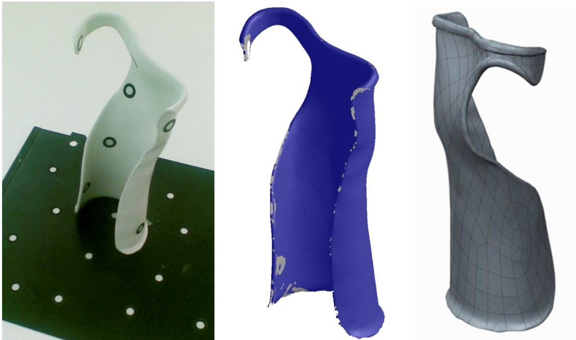
Figure 2. Reverse engineering process with the classic splint: reflective targets placed (left), geometry digitalised in ZScan (middle) and surface reconstruction with Geomagic Studio 2013 (right).
