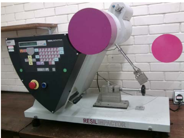
Fig. 1. Resil impact test set-up with GFRP specimen
