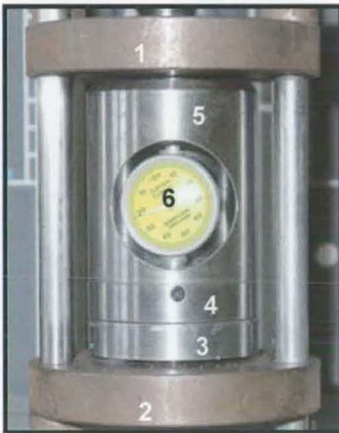
Fig. 7.06: Arrangement on the extensometer for the compaction-thickness tests
