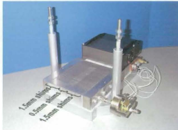
Fig 6.05 Segmented current collector piece
