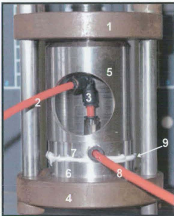
Fig. 7.30: Arrangement on the extensometer for the compaction-through plane pressure drop tests
