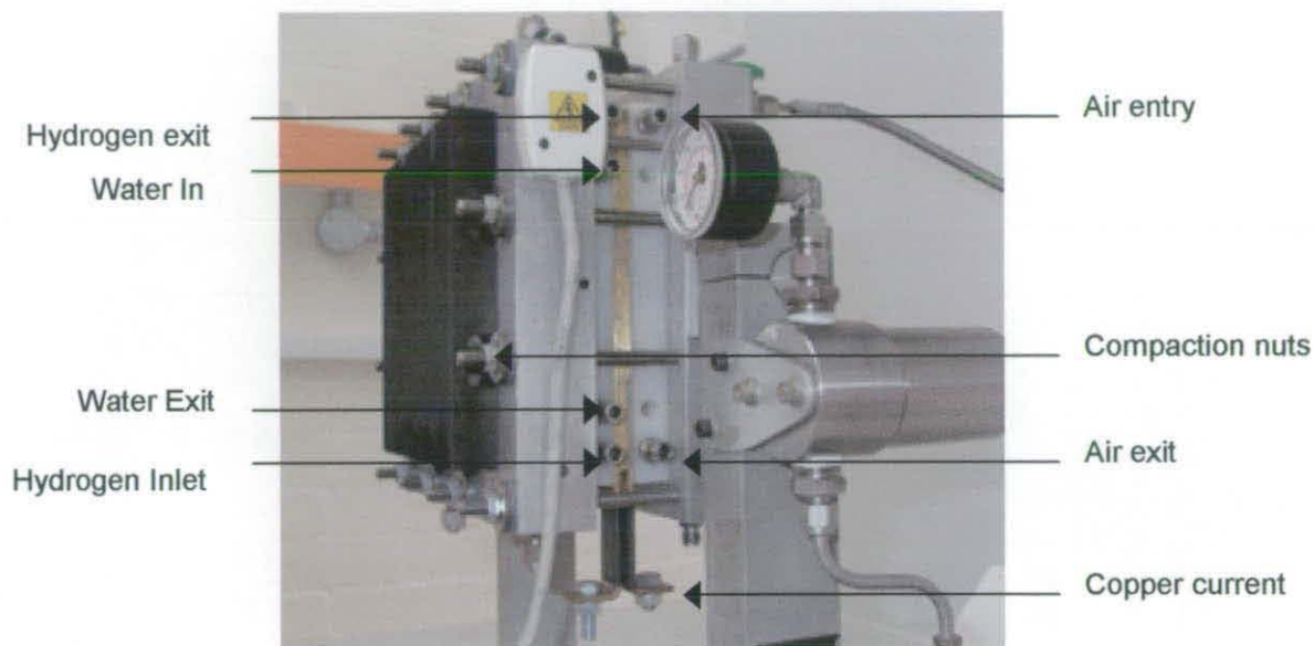
Fig. 3.13 Right hand view of FC rig
