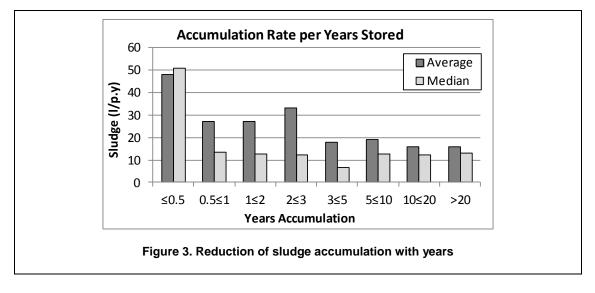
Never emptied systems had a lower sludge accumulation rate at 14 l/p.y compared with regularly emptied systems at 41 l/p.y, which accords with the above point, since and never emptied systems were an average 15 years old and regular emptying occurs after less than 2 years storage.
