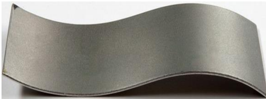
Figure 3-7 Double curvature metal plate
