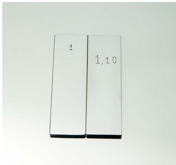
Figure 4-9 Slip-gauge arrangement to create a step-height of 100 \mu\text{m}
