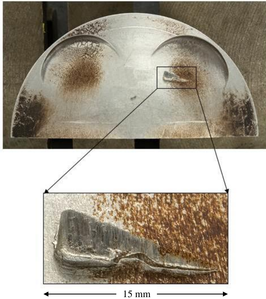
Figure 7-15 Surface defect (Defect ID – 4) embedded in the piston crown
