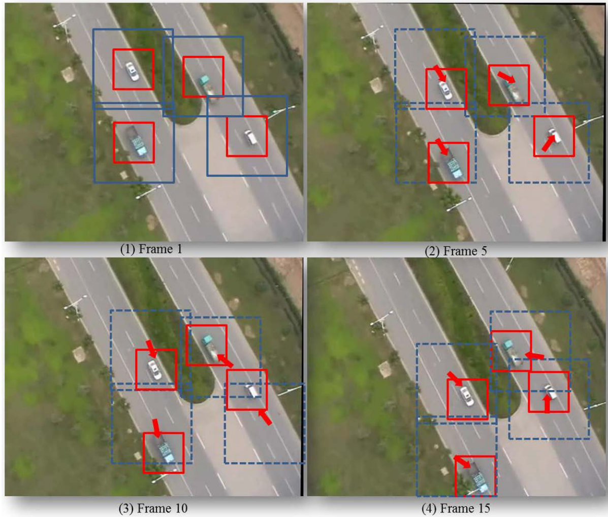
Figure 6.2: The detector process in a sequence of frames. The red boxes are the detectors that detected vehicles in the current frame. The blue boxes are the prediction areas in the following frame and the arrows are the moving factors of the detectors.
