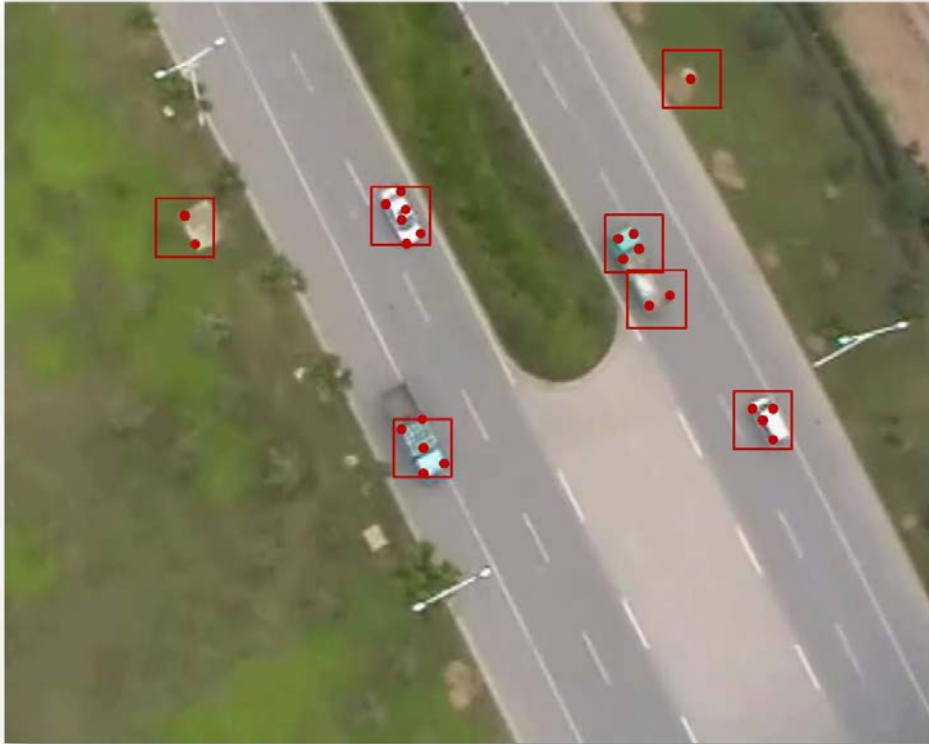
Figure 4.7: Examples of detection results using the SIFT feature approach.
