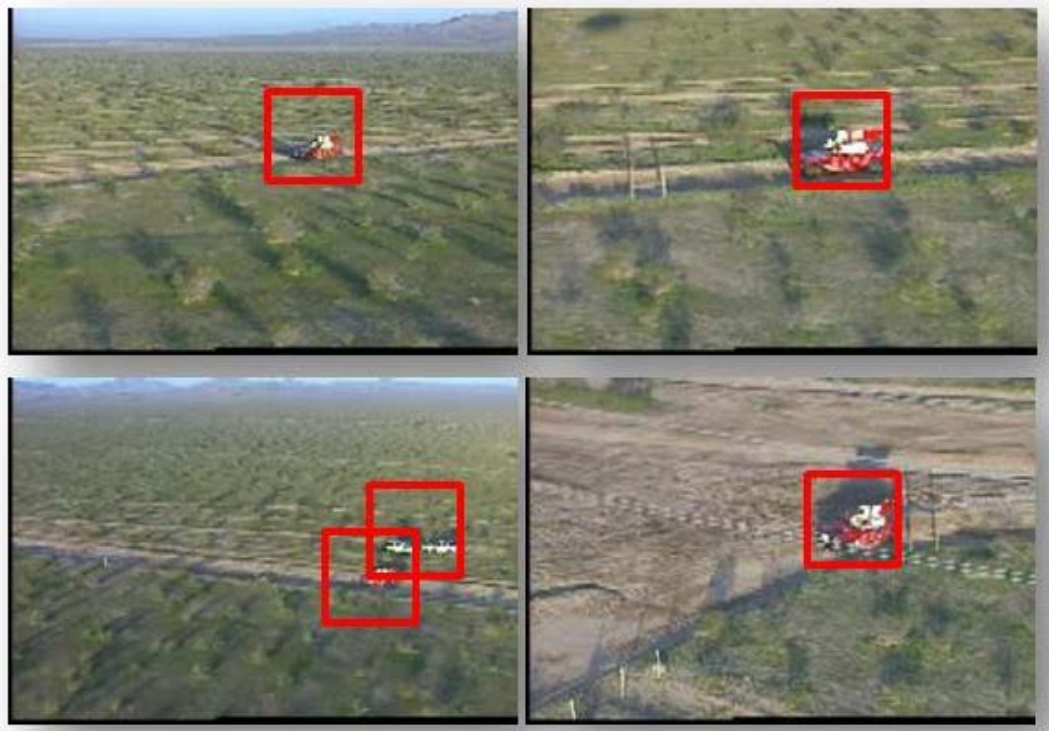
Figure 6.11: Tracking results from a situation in which the target changes appearance and size during tracking.
