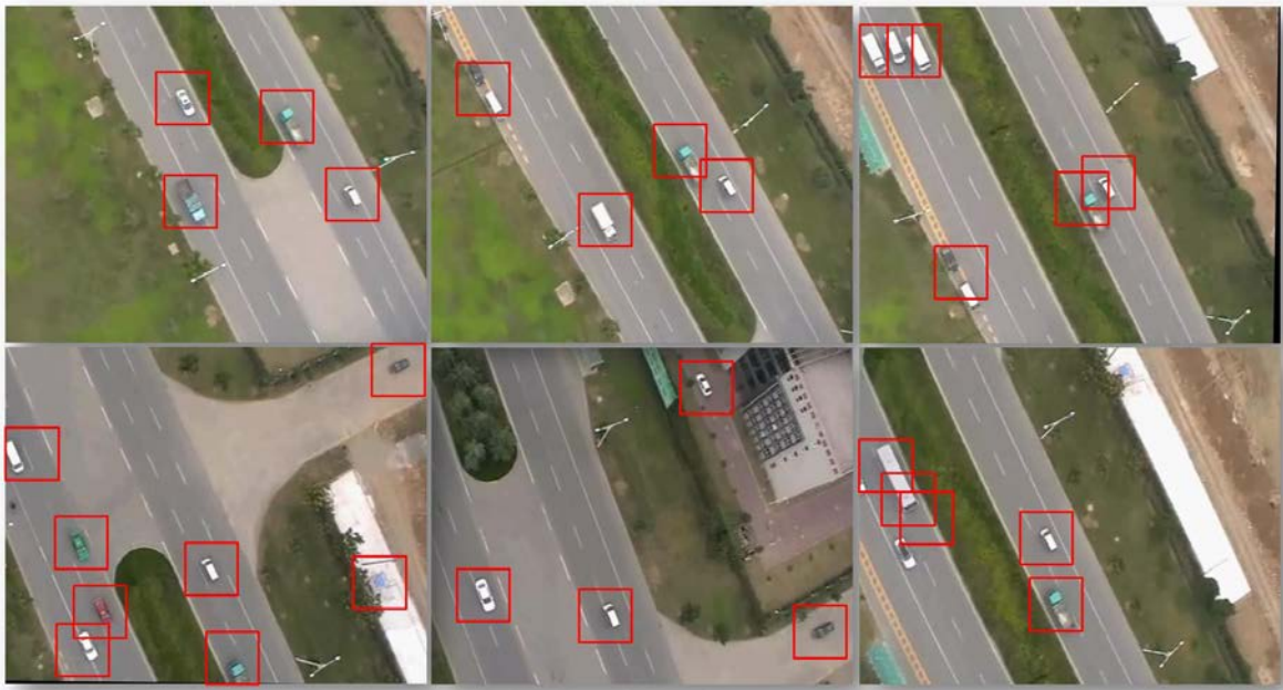
Figure 4.12: Examples of detection results using the ISM-SIFT detection approach.
