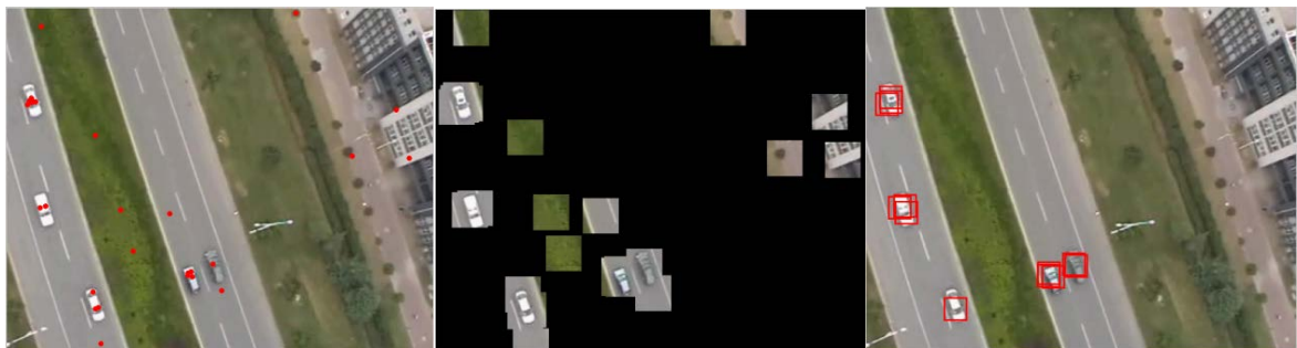
Figure 4.11: An example of the ISM-SIFT detection process. (Left: the SIFT point detection, Middle: codebook selections, Right: final detection)
