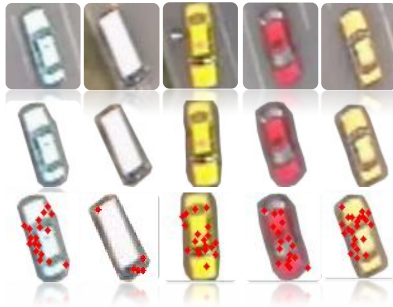
Figure 4.5: Examples of positive sample selections of SIFT points (First row: original sample images; second row: the background removal; third row: distributions of SIFT point's).
