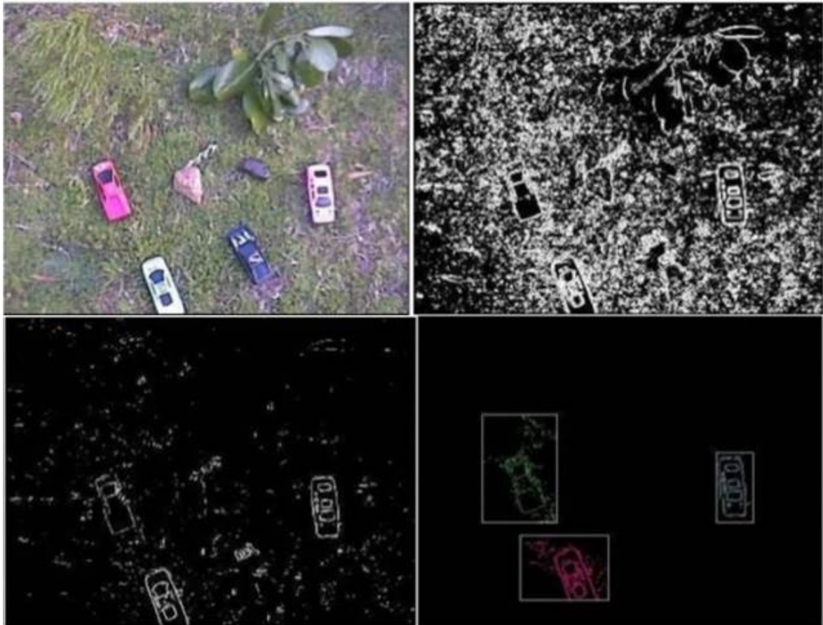
Figure 2.1: Examples of vehicle detection using edge features at different thresholds. The background noise can be removed in higher threshold detection. [22]
