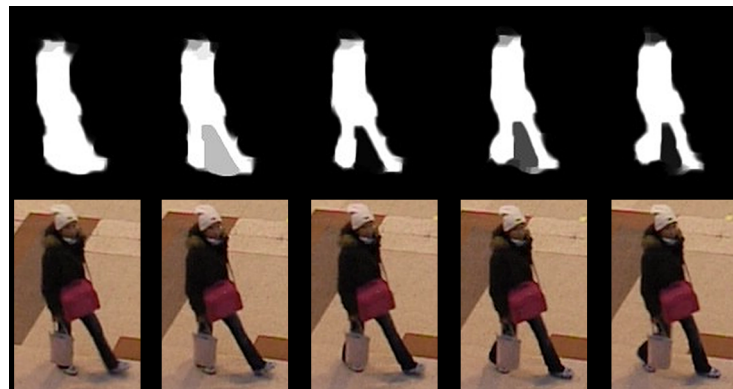
Figure 7.1: An example output of CFC algorithm where parts of the background are included into the foreground.
