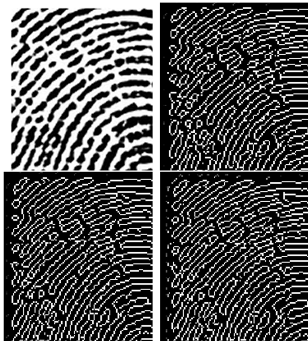
Figure 4.5: From left to right in first and second row: Fingerprint image convolved with the derivative of Gaussian filter, EEF and a \text{sinc}(x) filter and undergone non-maximum suppression with threshold 0.5.
