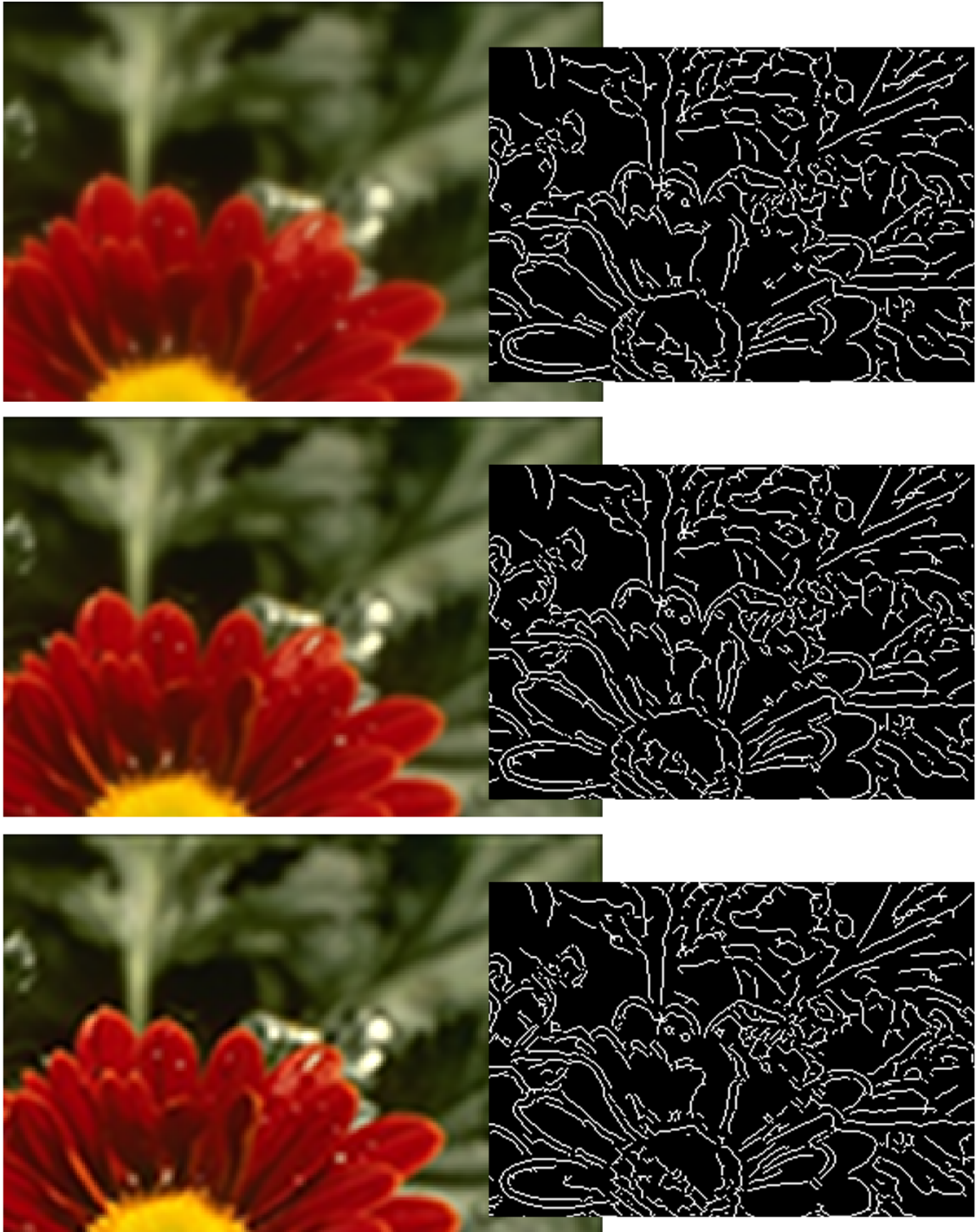
Figure A.2: flower image filtered with the Gaussian filter of \sigma = 1.5 , EEF filter and the \text{sinc}(x) filter. The size of all filters was 13 \times 13 sampled in the interval [-2\pi, 2\pi] . The corresponding edges are obtained after non-maximum suppression with threshold 1.3 and hysteresis thresholding with thresholds \text{thresh}_{high} = 0.5 and \text{thresh}_{low} = 0.01 .
