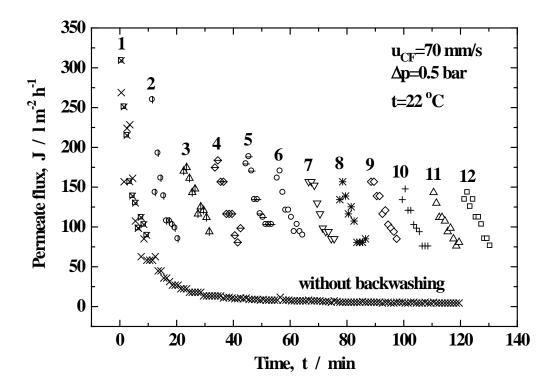
Figure 7. A comparison of permeate flux fluctuations with time during MF without and with air backwashing for 1 min every 10 min. The gauge pressure of air during backwashing was 0.5 bar.
