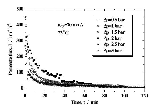
Figure 5. The variation of permeate flux with time at different transmembrane pressures for MF of red raspberry juice at 22 °C and cross flow velocity of 70 mm/s. The permeate was recycled back to the holding tank to keep VCF = 1.
