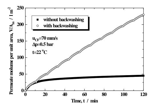
Figure 8. The permeate flux collected per unit membrane area as a function of time during MF of red raspberry juice without backwashing and with air backwash every 10 min for 1 min. The gauge pressure of air during backwashing was 0.5 bar.
