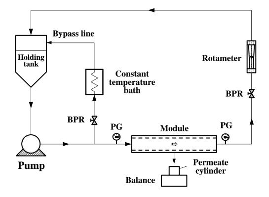
Figure 2. Schematic diagram of microfiltration/ultrafiltration rig used in this work (PG – pressure gauge, BPR – back-pressure regulator).
