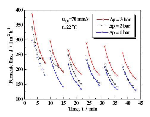
Figure 9. The variation of permeate flux with time at three different transmembrane pressures during MF with air backwashing. The membrane was backwashed with air at the gauge pressure of 0.5 bar every 6 min for 1 min.
