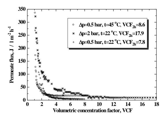
Figure 6. The permeate flux as a function of volumetric concentration factor at different transmembrane pressures. The volumetric concentration factor obtained after 2 h (VCF<sub>2h</sub>) at different operating conditions was indicated in the legend. The initial volume of the juice was 8.5 l.
