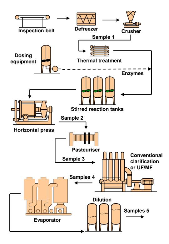
Figure 1. A scheme of the manufacturing process used in this work for red raspberry processing in clear juice concentrate using conventional clarification or membrane filtration (MF or UF). A light transmittance at 625 nm in samples 4 and the amount of total anthocyanins in samples 1 to 5 are given in Figures 3 and 4, respectively.
