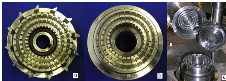
Figure 3 Ytron Z-Lab (a) rotor with pumping wheel; (b) stator; (c) mixing head
