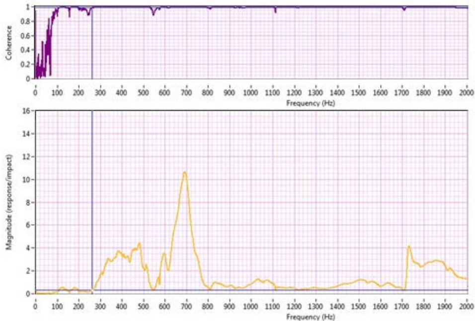
Figure 4 Static FRF impact tests: an example of the measured FRF with the acceleration amplitude at the bottom and the corresponding coherence at the top.
