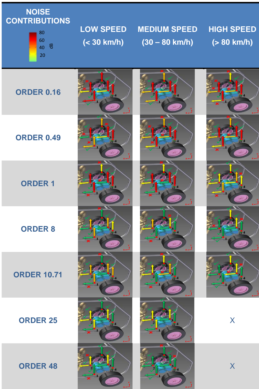
Figure 22 Contribution of each path (1 to 8) calculated using the TPA and agreement (✓) and discrepancies (✗) with the corresponding OPA result at the dominant engine orders in the low, medium and high frequency ranges.
