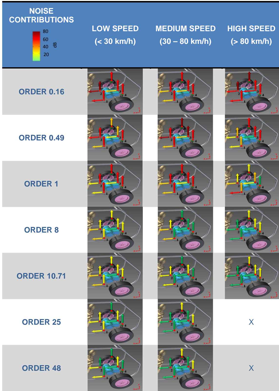
Figure 15 Summary illustrations of the relative strength of each path (1 to 8) calculated using OPA at the dominant engine orders in the low, medium and high speed ranges.
