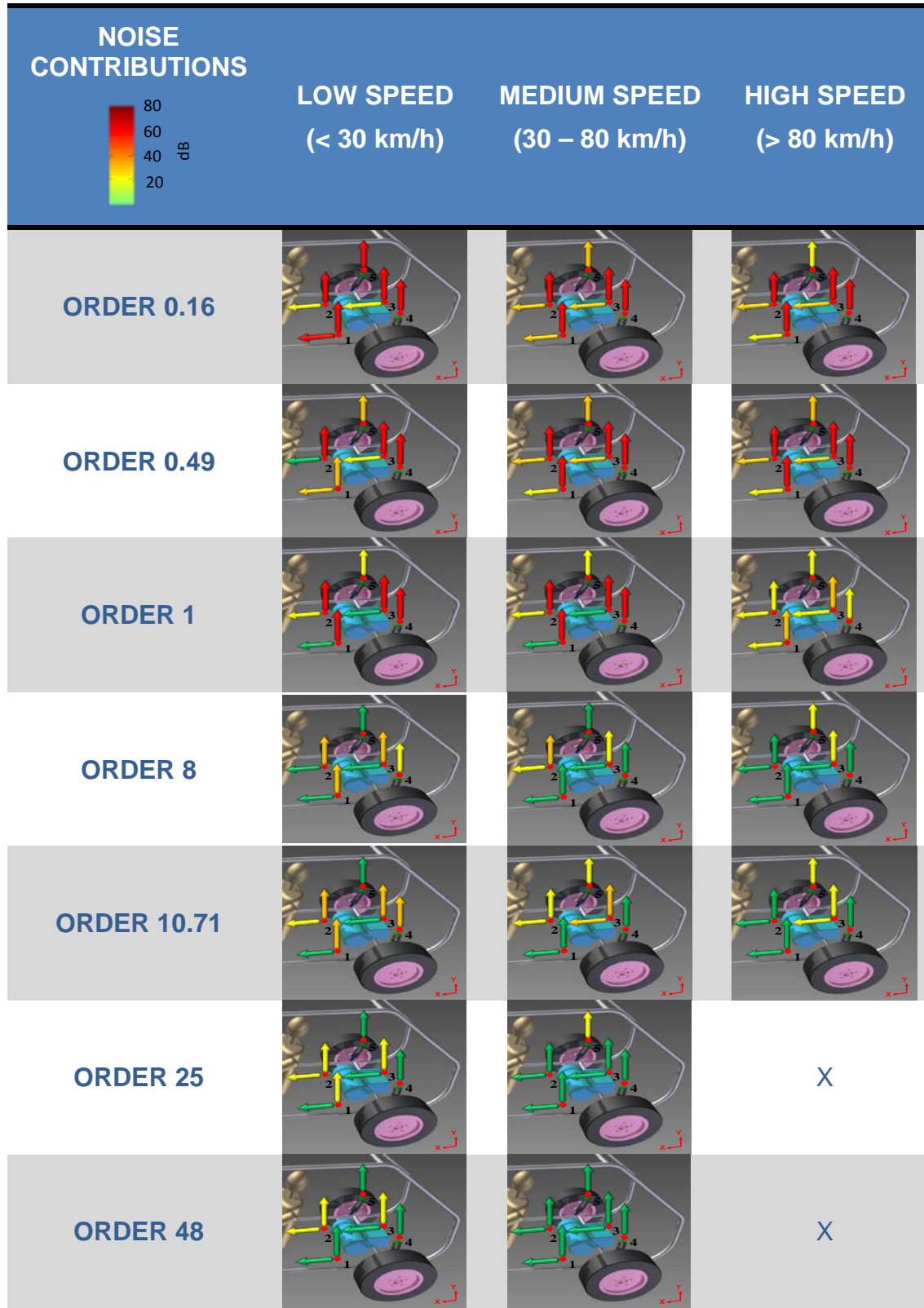
Figure 21 Summary illustrations of the relative contribution of each path (1 to 8) calculated using the TPA at the dominant engine orders in the low, medium and high speed ranges.
