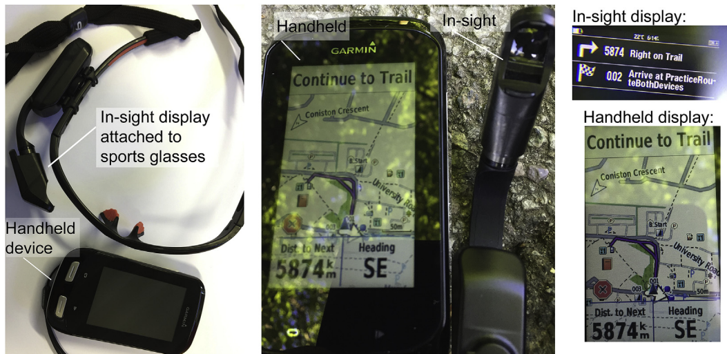
Fig. 2. Left: in-sight display attached to glasses (top), handheld unit (bottom). Middle: relative size of units. Right: illustration of instructions as shown on in-sight display (top) and handheld (bottom).
