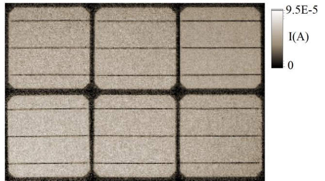
Fig. 5. CS current map of the 6 cell PV module used in these experiments. The CS current map is produced having acquired 30000 (50%) of measurements.
