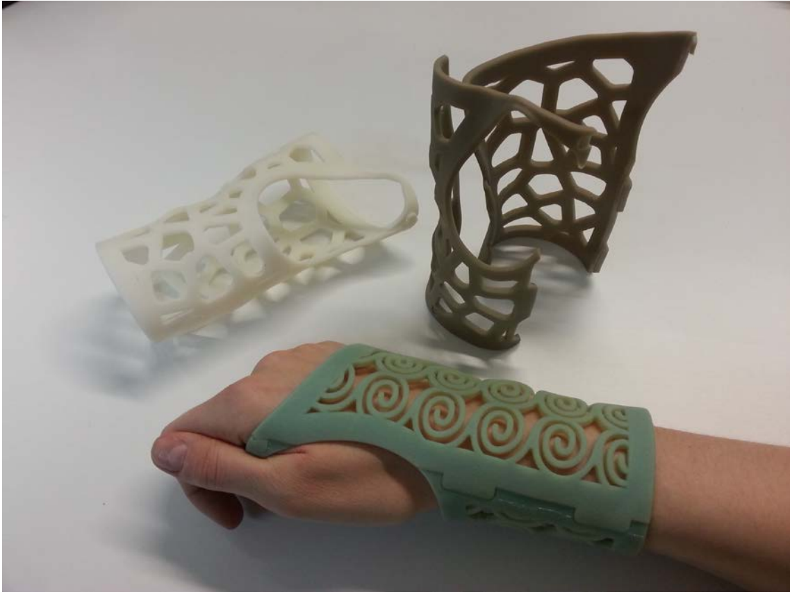
Figure 7: Proof-of-concept AM wrist splint prototypes
