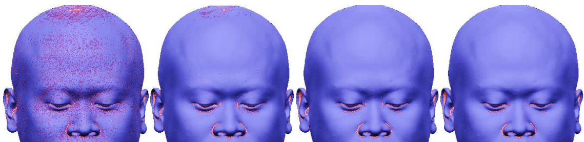
Figure 36: Thresholded mean curvature map at (a) 0-ring, (b) 1-ring, (c) 5-ring and (d) 10-ring neighbourhood averaging filter sizes
