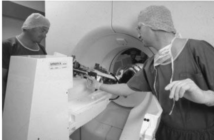
Figure 6: 'Minerva' neurosurgery robot 7
