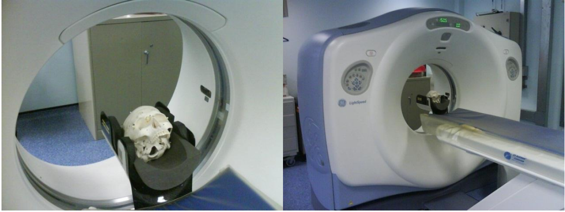
Figure 20: CT scanning of the anthropomorphic skull with radiopaque markers attached
