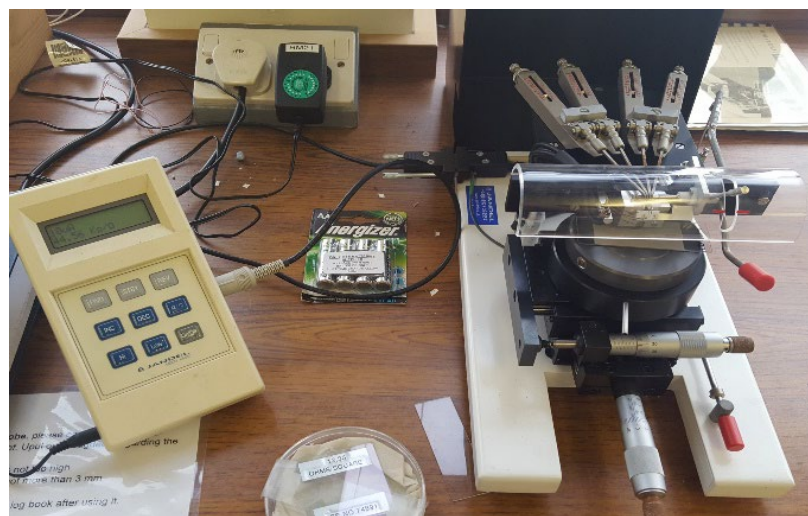
Figure 40 Four Point Probe measurement of sample
