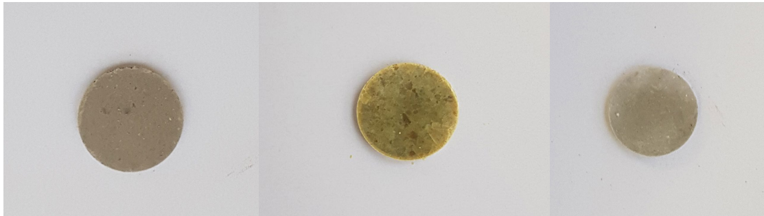
Figure 51 Microwave sintered metal oxide pellets
