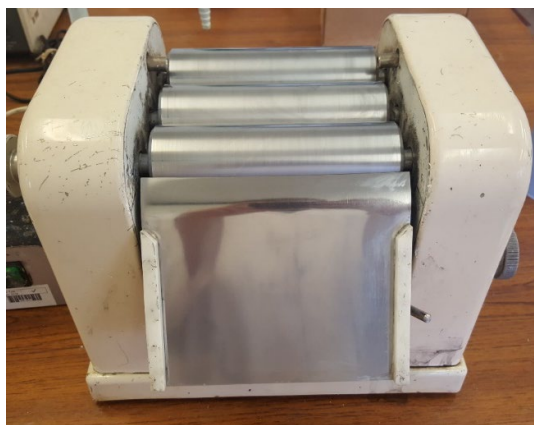
Figure 39 EXAKT Three Roll Mill to be used
