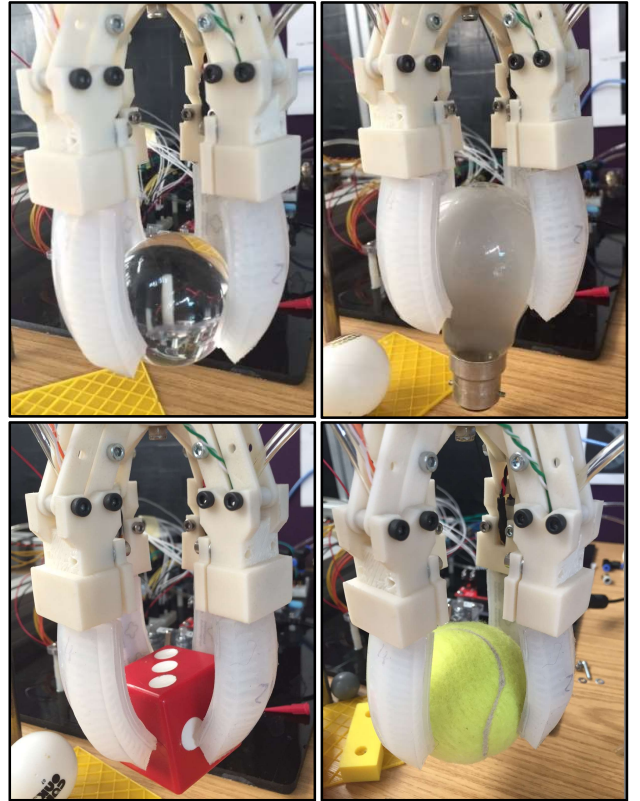
Figure 2: Sample images for grasping tests showing the soft gripper successfully grasping a small sphere, light bulb, dice and a tennis ball.
