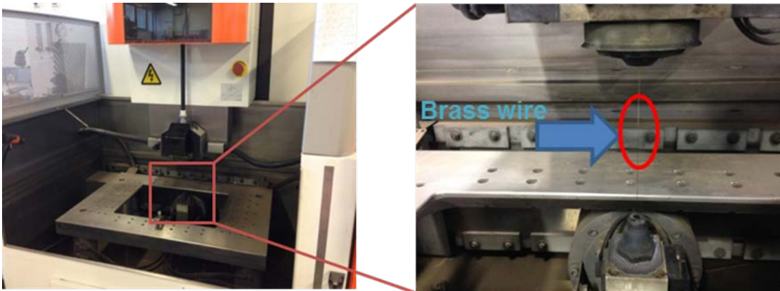
Figure 3-10 Micrograph of EDM with brass wire employed to prepared wedge indentation specimens.
