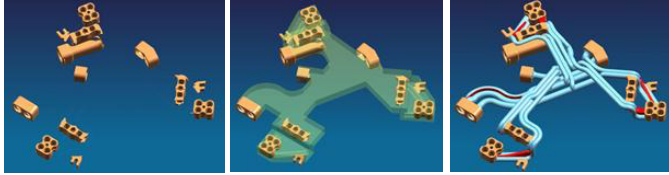
Fig. 57. Manifold designed from the bottom up for AM starting with the interfaces (left), defining the maximum envelope as a constraint (center), and then adding functional features and reinforcement (right). Courtesy of ASML.
