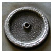
Fig. 32. Functionally graded flywheel (outer radius 0.2m) composed of 320 stainless steel and copper coated nickel produced using the LENS process [233].
