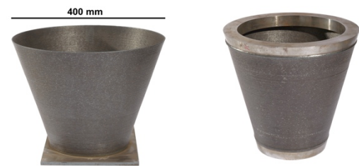
Fig. 52. Truncated cone produced in mild steel by Wire + Arc Additive Manufacturing: as printed (left, courtesy of the Welding Engineering and Laser Processing Centre at Cranfield University) and welded (right, [352]).
