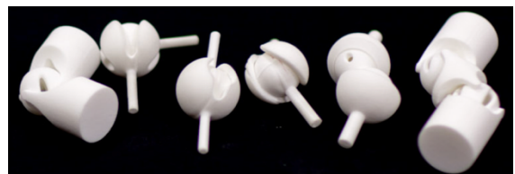
Fig. 35. Articulated joints produced using selective laser sintering (SLS) [55].
