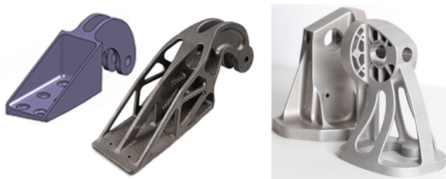
Fig. 16. Brackets before and after topology optimization: Airbus A320 nacelle hinge brackets as-designed for cast steel and optimized for titanium (left) and Airbus A380 brackets as designed and optimized for stainless steel [105]. The optimized brackets were produced by direct metal laser sintering (DMLS).
