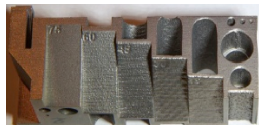
Fig. 38. Benchmark showing the surface roughness resulting for SLM parts with different build angles. Courtesy of ASML.
