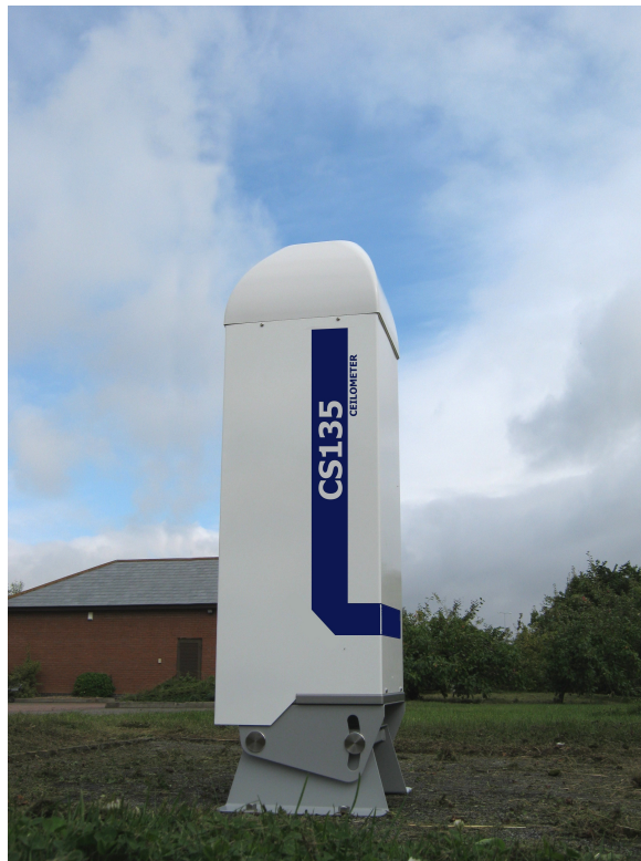
Figure 3.26: Prototype instrument in full external enclosure with cowelling.
