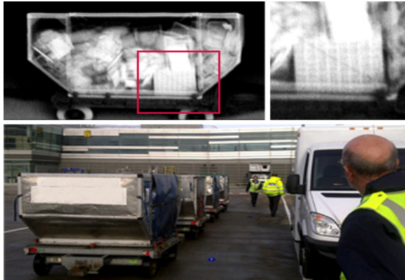
Figure 2.6 Back scatter technology revealing smuggled cigarettes (in red box). (Image courtesy American Science and Engineering, Inc.)
