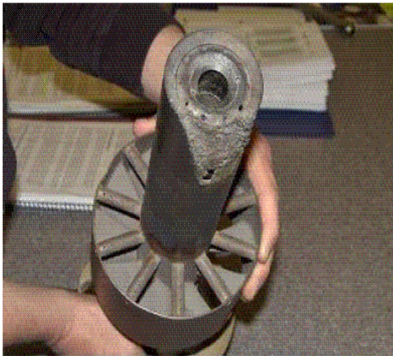
Figure 1. 4 - Damage to a GE- 7EA (80 MW) fuel nozzle due to combustion dynamics, (Lieuwan et al. 2003).
