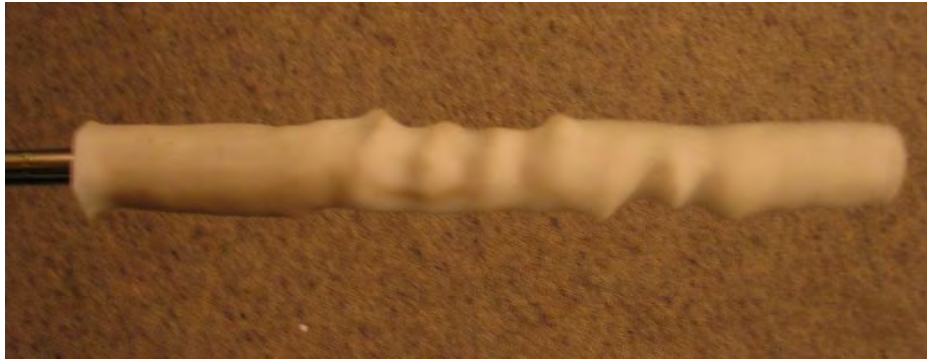
Figure 88: Customised AM Golf Club Grip. Source: Olaf Diegel, Auckland University of Technology, New Zealand.
