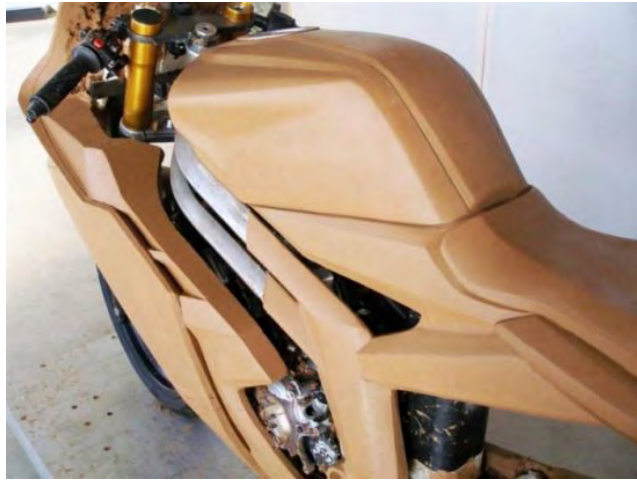
Figure 28: A design development model made with clay of a motorbike. Source :< www.coroflot.com > 25/10/10
