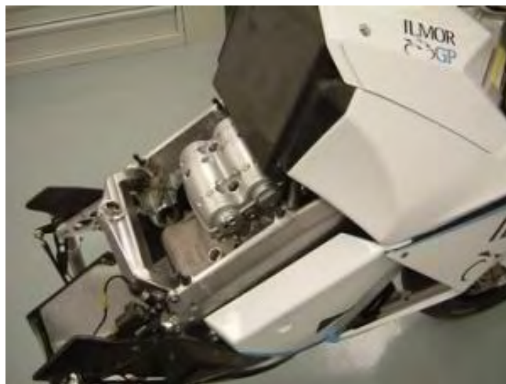
Figure 62: Structural parts of a motor produced with laser sintering (in white) Source: < http://www.engineerlive.com/ 12/03/09
