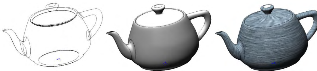
Figure 70: CAD visualisation, wireframe (left), solid & surface model (middle), photorealistic image (right)
