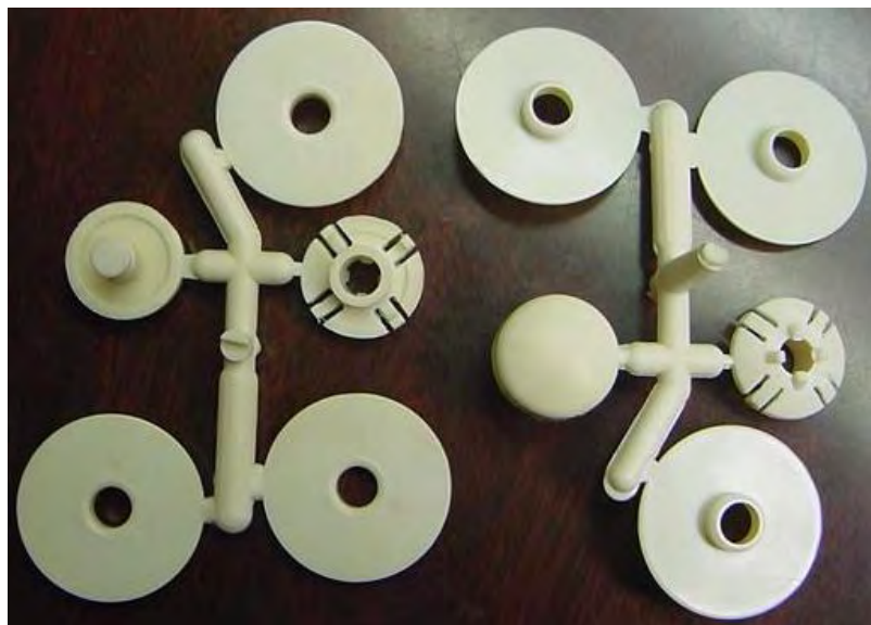
Figure 37: Off-tool prototype for a consumer product Source :< http://www.prototypingrapid.com/page/1042348 >27/10/10
