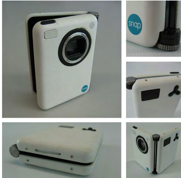
Figure 31: An appearance prototype of a camera. Source :< http://nicmarks.com/ > 26/10/10
