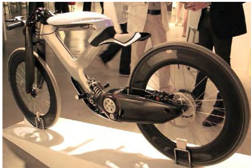
Figure 30: A functional concept model of a motorcycle. Source :< www.illusion.scene360.com > 26/10/10
