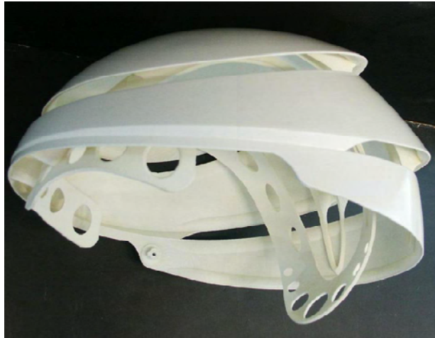
Figure 68: Personalised sports-helmet manufactured using Laser Sintering. Source: < http://tno.nl/index.cfm > 12/03/09
