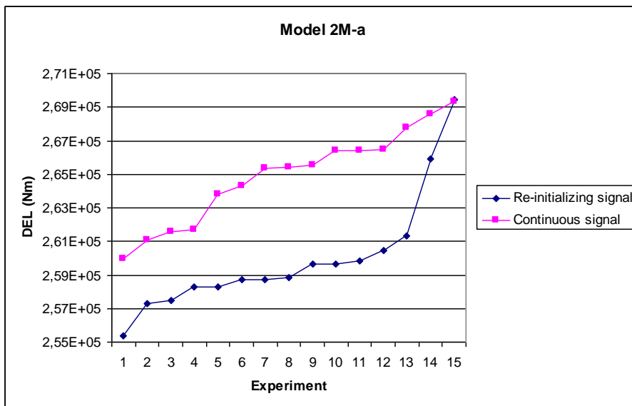
Figure 49: Performance of the top 15 DTDs for the Model 2M-a wind turbine, as they were tuned using experiments run with the re-initialized chirp signal and experiments run with the continuous signal.
