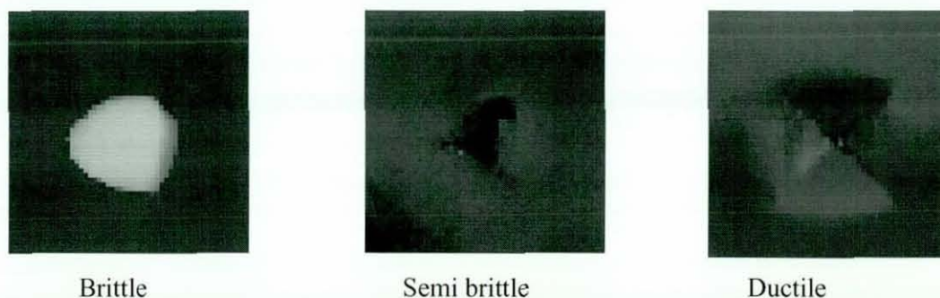
Figure 6.18 Impact failure modes under impact loading
