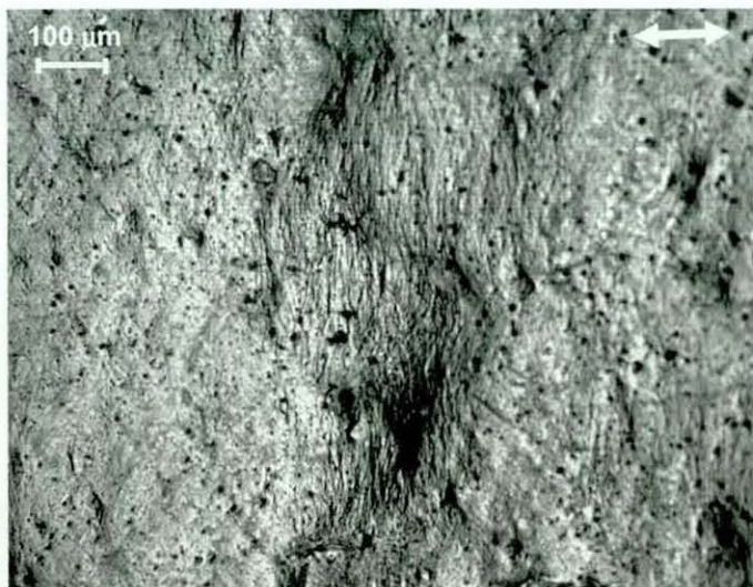
Figure 6.10 Optical microscopic image of stress cracks on the surface of a 50:50/3H/0.6D blend tensile fractured specimen
