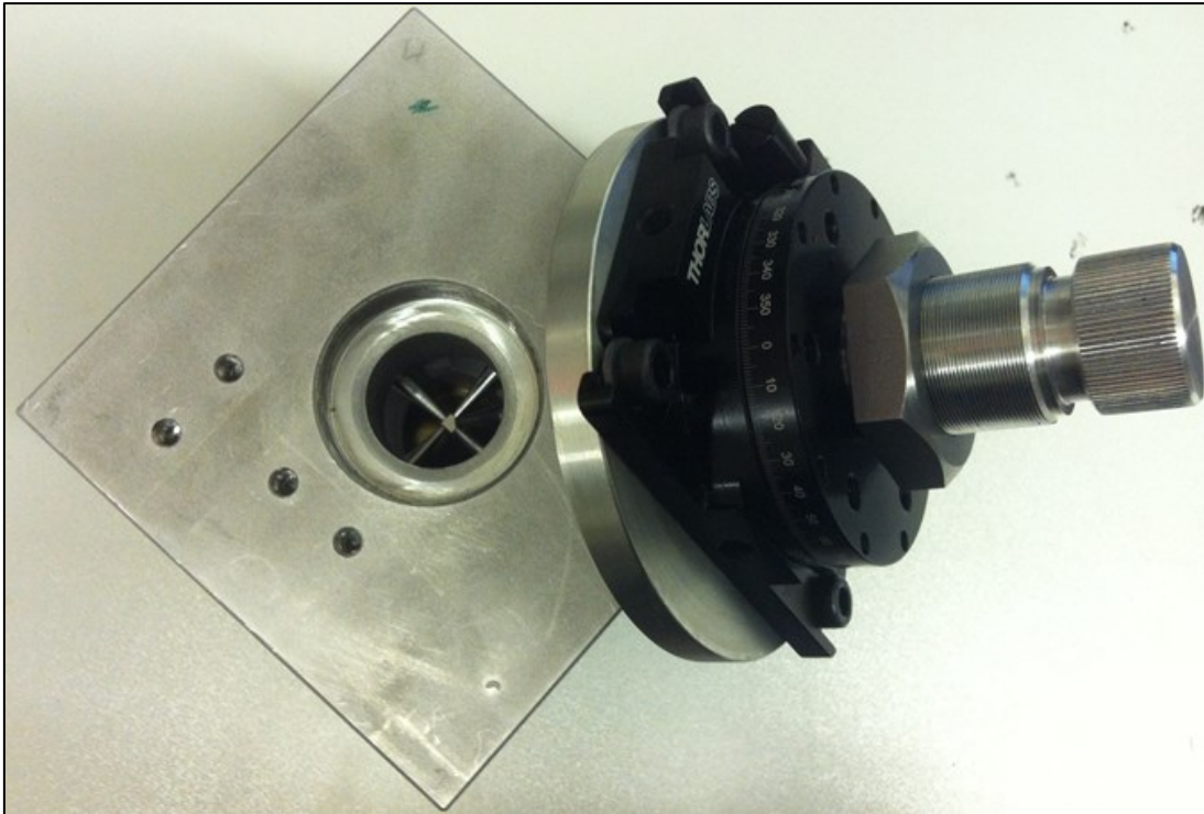
Figure-3.12: Manufactured assembly of the calibration artefact positioning device.
