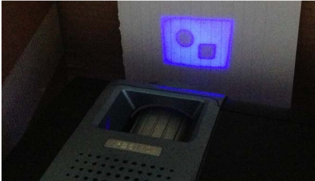
Figure 3.8. Projected UV image from DLP projector
