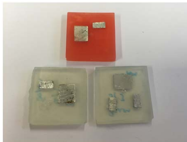
Figure 6.24. Embedding in MakerJuice SF Resin without stress cracking
