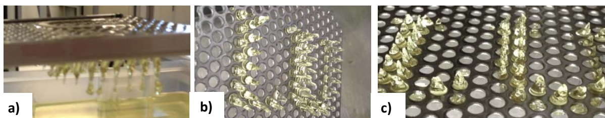
Figure 3.16. Trials conducted with a) 9000 \text{mJ}/\text{cm}^2 , b) 4500 \text{mJ}/\text{cm}^2 and c) 900 \text{mJ}/\text{cm}^2 energy doses per layer
