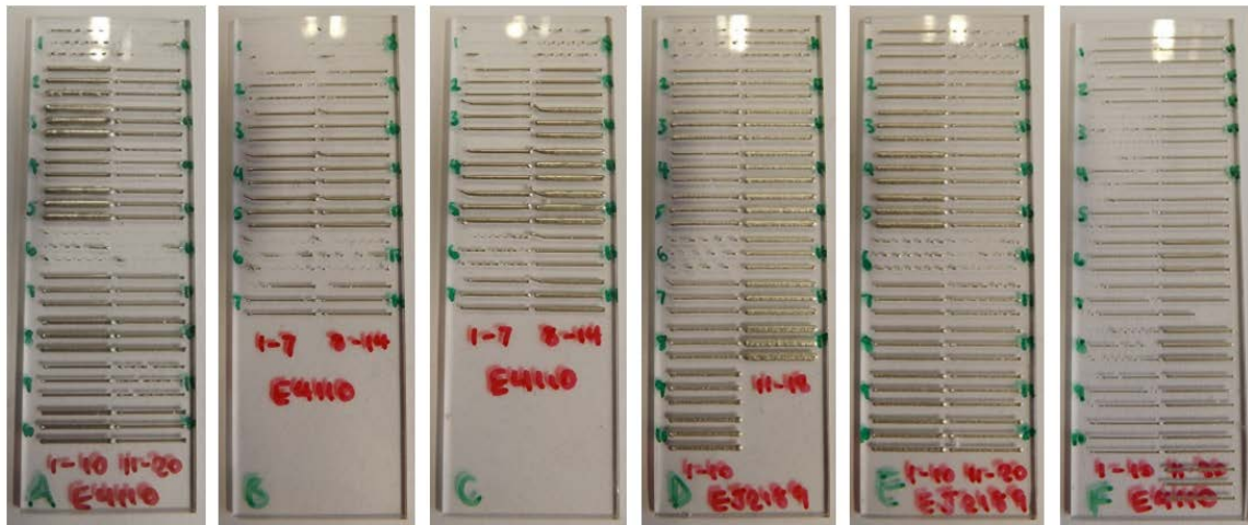
Figure 5.11. Array of cured tracks dispensed during process characterisation through all three nozzles in materials A and B
