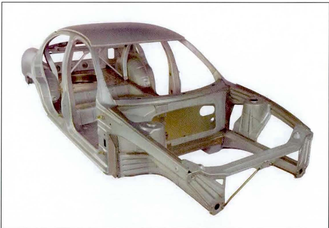
Figure 5: The UltraLight Steel Auto Body (ULSAB)
