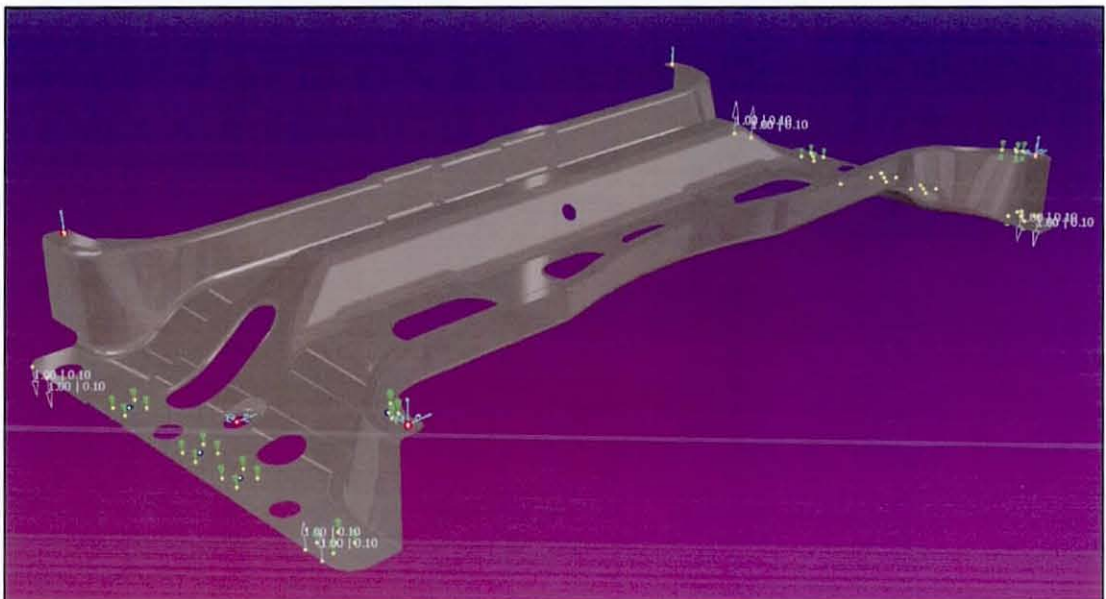
Figure 45: Crossmember with input deviations represented by white arrows
