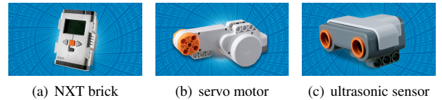
Fig. 9. NXT components used in the testbed (thanks to http://mindstorms.lego.com/ )
