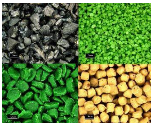
Figure 2.3. Example of different types of rubber / polymers infills available for 3G artificial turf. Styrene-butadiene-rubber (upper left) is most commonly used, but specially developed infill (upper right and lower left and right) are also available.
