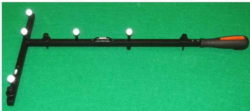
Figure 7.10. Calibration wand used for both the static and dynamic calibration of the Vicon 3D motion capture system.
