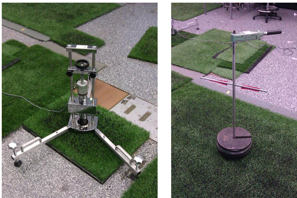
Figure 7.7. The advanced artificial athlete (AAA) and rotational traction device used for measurements on the hardness (force reduction) and rotational traction properties of the surfaces
