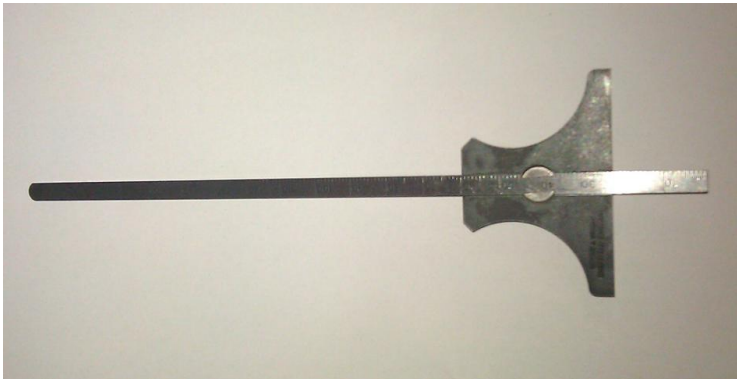
Figure 6.3. Depth gauge meter used to measure the infill depth. The base was pushed through the infill to the backing of the carpet after which the top (black) was slid down to the top of the infill to determine the infill depth
