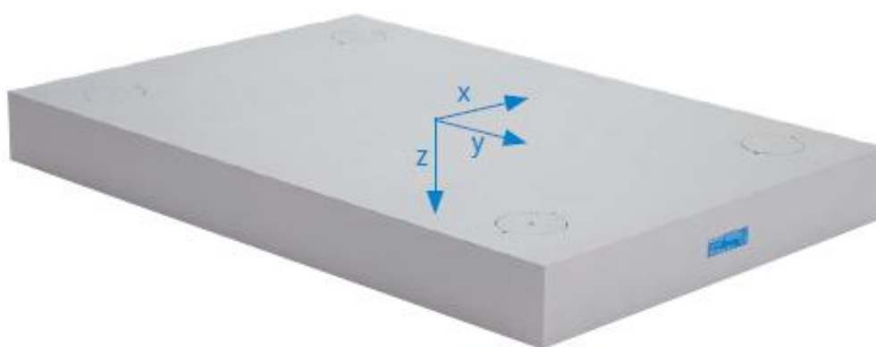
Figure 7.5. Kistler 9287 BA force platform including the force coordinates: z (vertical), y (anterior / posterior), x (medial / lateral)
