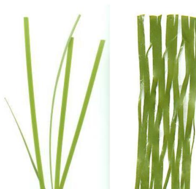
Figure 2.2. Example of different types of fibres used in the carpet of artificial turf surfaces, monofilament (left) consist of single fibres, whereas fibrillated (right) fibres are at first connected to each other and split during use.
