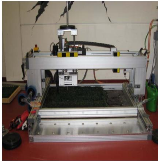
Figure 2.13. Test device developed by Adidas as used in a study by Severn (2010) to measure the rotational traction of the shoe-surface interface
