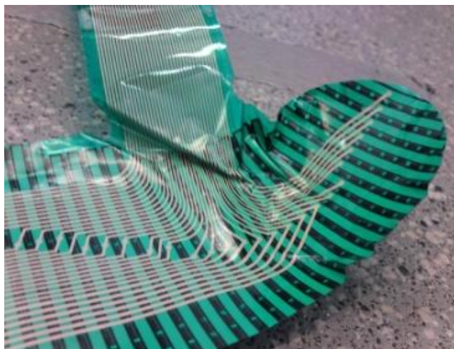
Figure 5.7. The pressure insole was deformed as a result of a shift inside the shoe of the subject during the 24 minute run. The deformation mainly took place around the cuff and the heel area of the insole.
