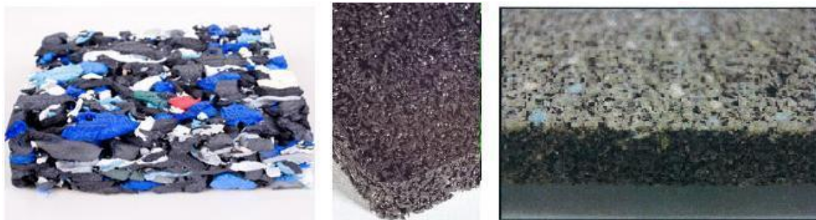
Figure 2.4. Example of different types of pre fabricated shockpads available for 3G artificial turf made from rubber (middle), closed-cell foam (right) and a mixture of different foam products (left).
