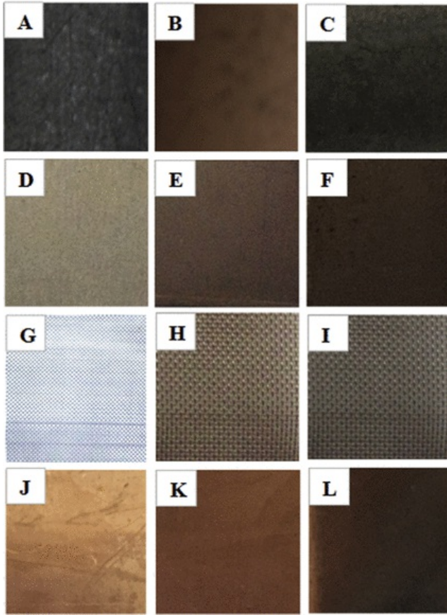
Fig. 6 Naked eye observation on CR (A, B and C), TS (D, E and F), SSM (G, H and I), and CS (J, K and L) cathodes. Fresh bare cathode (A, D, G and J) after the first cycle (B, E, H and K) and the subsequent exposure to air for 48 h (C, F, I and L).
