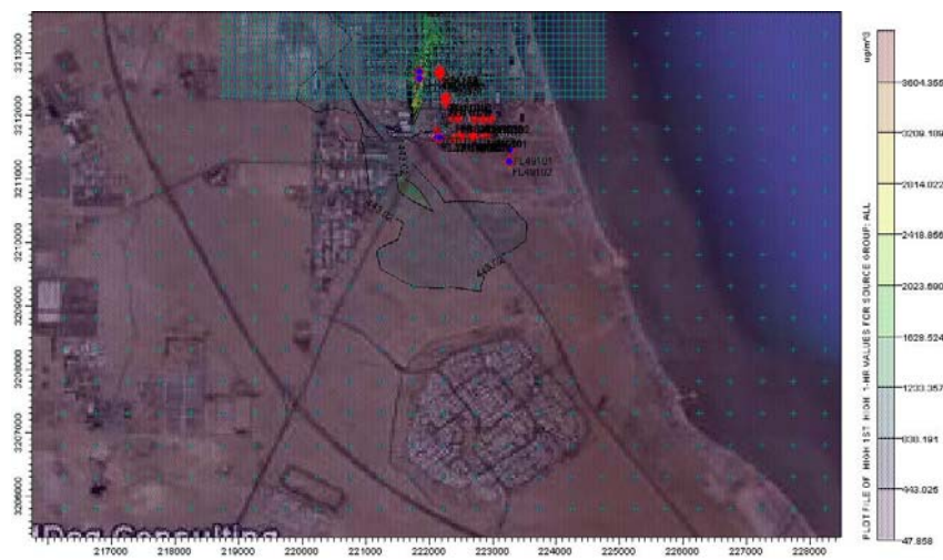
Figure 5.9: AERMOD plume output results for CO Hourly concentration. (Umm-Alhyman Area at the South)
