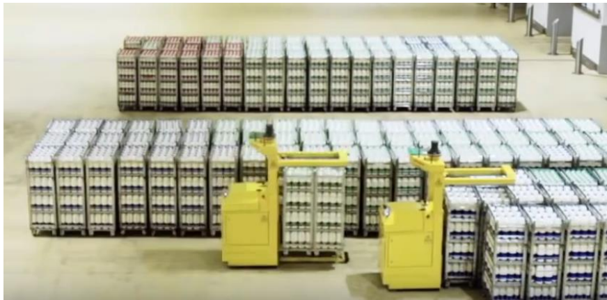
Figure 9.1 No interruption caused by other AGVs [120]
