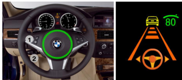
Figure 6.3: Peripheral light display indicating that the lateral component of a traffic jam assist is activated (Schaller, Schiehlen and Gradenegger 2008)
