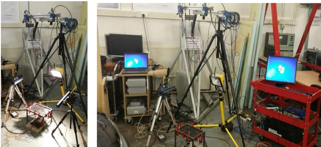
Fig. 5 – Photograph of the DIC setup between the camera and plate with the additional lamp. Fig. 6 – Photograph of the complete setup between the DIC equipment and Photon setup.
