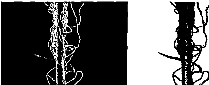
Figure 5-53 (a) A dark field yarn image (b) (a) after applying a threshold @25
