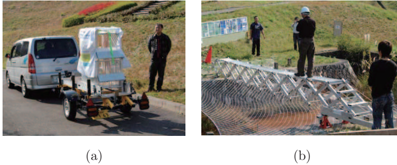
Figure 2: Pedestrian type of MB using scissors mechanism in its structural form. (a) Store condition. (b) In service state.
